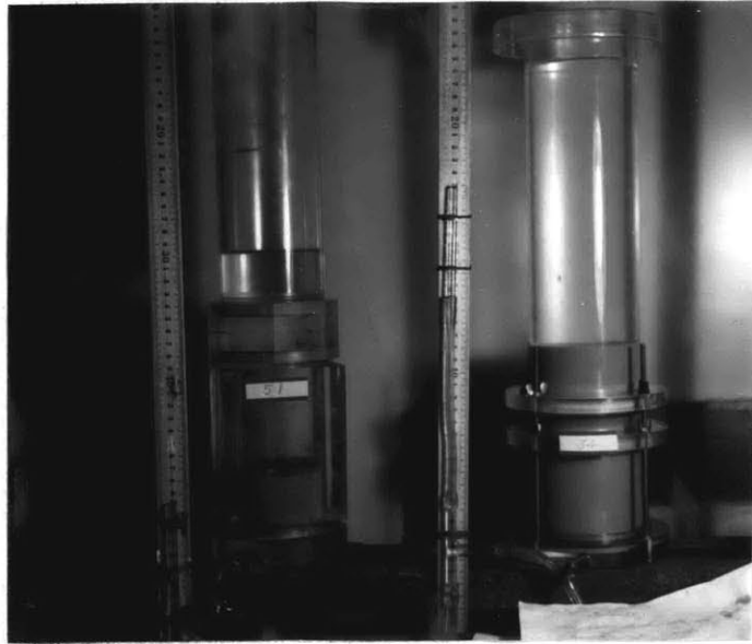
Photograph of sedimentation chambers
