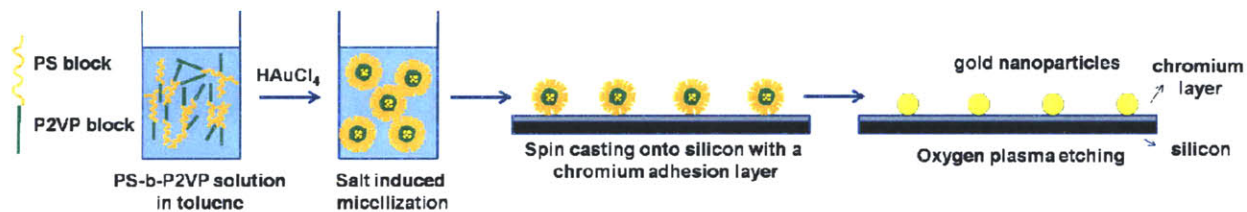
Scheme 3.2. Schematic illustration of gold nanoparticle array fabrication
