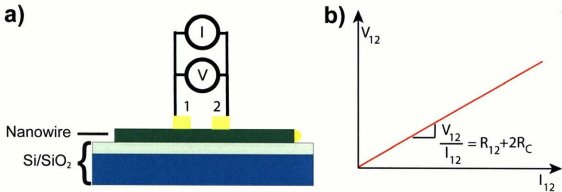
Figure 2-10: a) Schematic of nanowire two-point measurement. b) Expected IV curve and physical meaning of measured resistance
