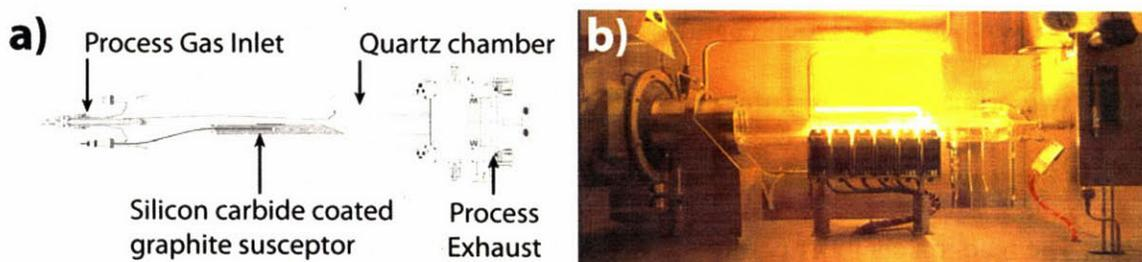
Figure 2-2: a) Schematic of MOCVD reaction chamber. b) Picture of chamber during operation.
