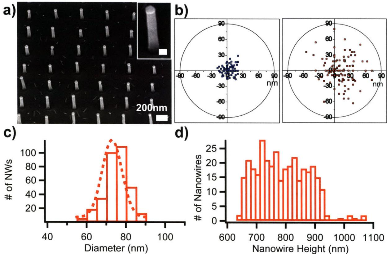
Figure 3-17: a) SEM image of an optimized vertical GaAs nanowire array. Distributions of the b) positions, c) diameters, and d) heights the nanowires grown from the Au nanoparticle array shown in Figure 3-6.
