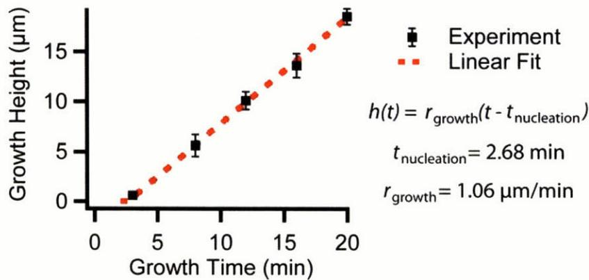
Figure 3-16: Growth rate calculation for GaAs nanowire growth.
