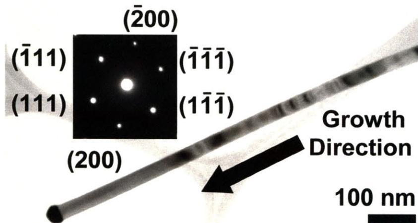
Figure 3-12: Bright-field TEM of GaAs nanowire with SAD pattern, (01-1) zone axis.
