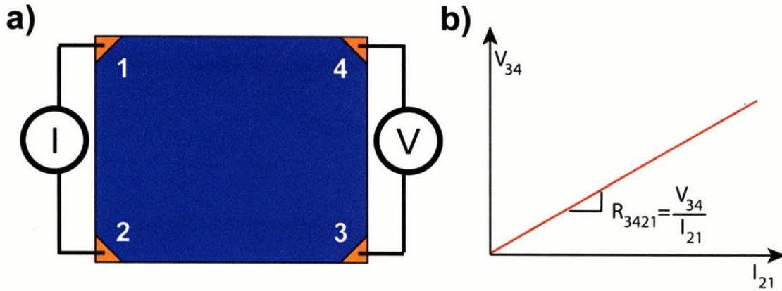
Figure 2-9: a) Schematic of thin film sheet resistance measurement using the Van der Pauw method. b) Expected IV curve
