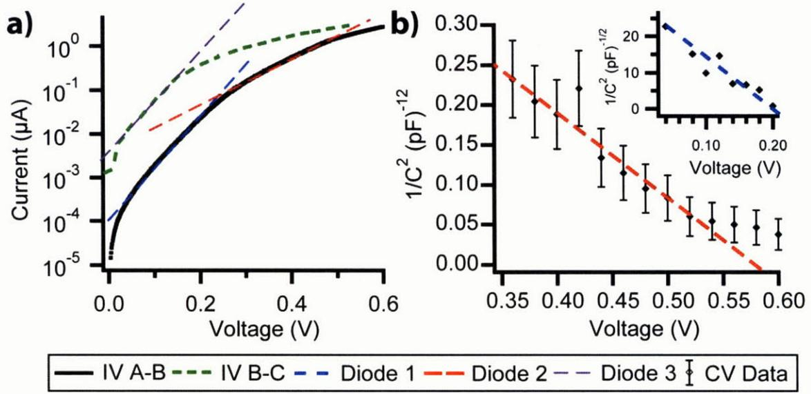
Figure 5-5: Electrical characterization between contacts A & B showing a) direct-current I-V behavior and b) C-V profiling using an AC bias of 500 mV at 1kHz. Inset is same data in a different voltage region and scaled accordingly.
