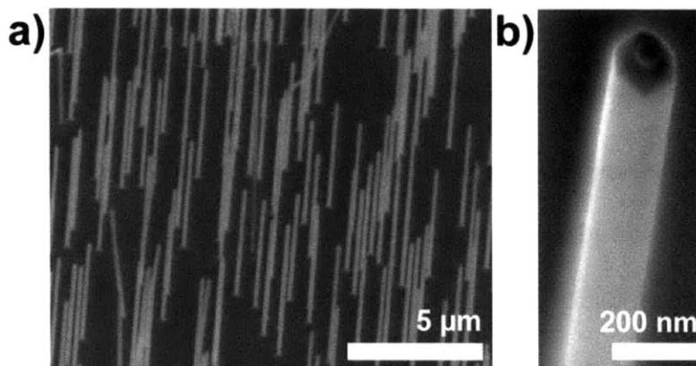
Figure 4-3: SEM micrographs of vertical core-shell nanowires showing a) 80 - 90% of nanowires maintain a stable morphology and b) the shell is faceted with a hexagonal cross-section.
