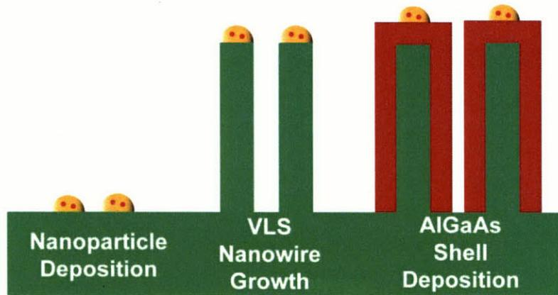
Figure 4-1: Schematic showing the shell deposition process.
