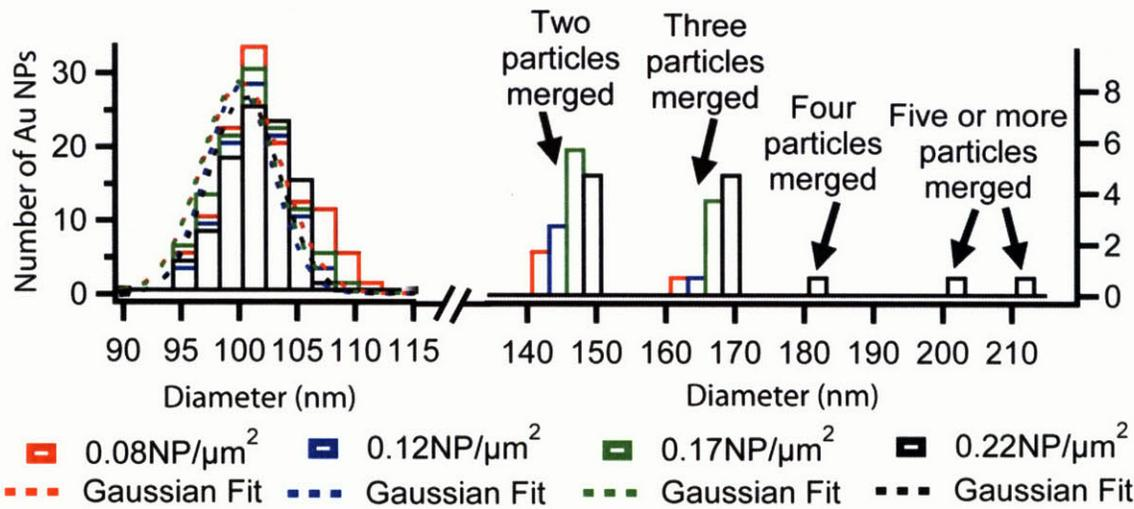
Figure 3-5: Diameter distributions of Au nanoparticles on GaAs 111B substrates at different aerial catalyst densities after annealing at 600°C for 10 min. The left and right histograms show the same data over different diameter ranges.
