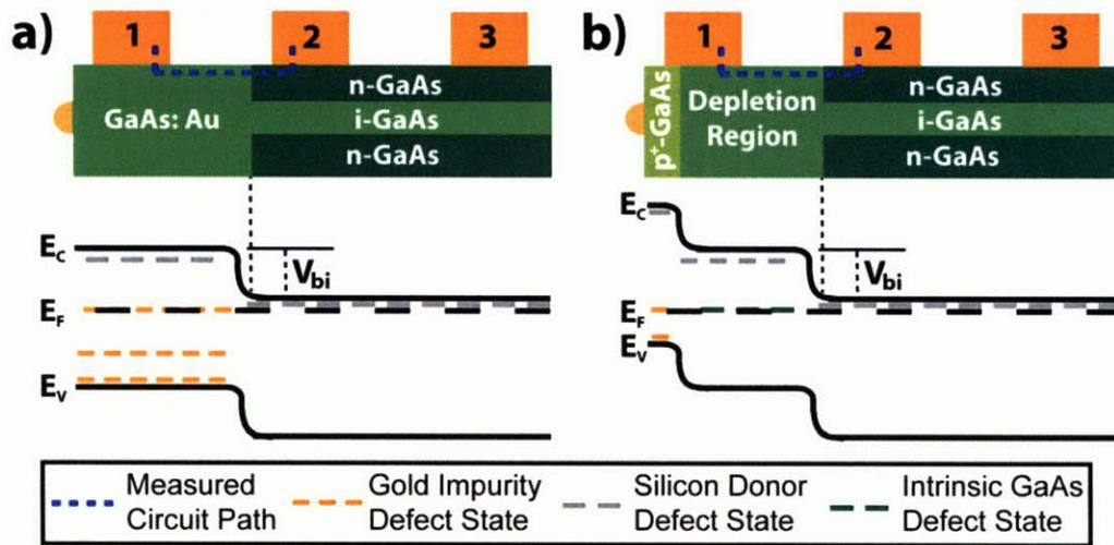
Figure 5-9: Proposed models for rectification. a) Au diffusion creates midgap states with observed rectification between Si- and Au-doped segments. b) Au diffusion creates degenerately p-doped region with observed rectification between the n-GaAs and diode depletion region.
