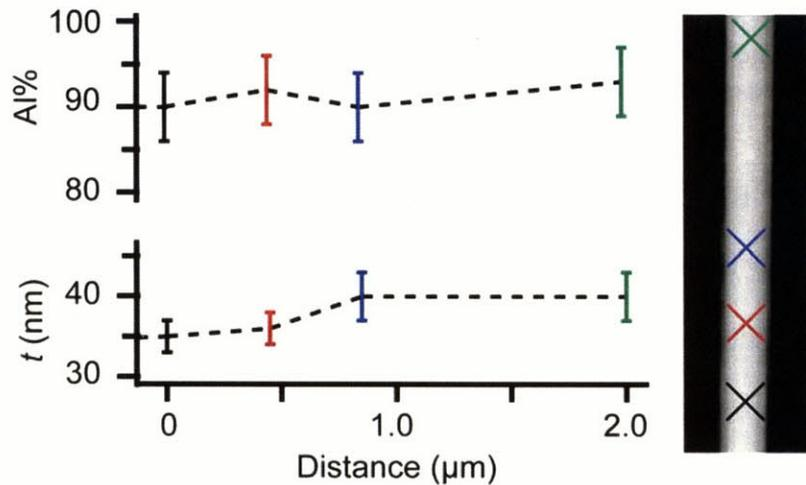
Figure 4-8: The shell composition and thickness of a representative core-shell nanowire measured by EDX at different point along the length of the nanowire.
