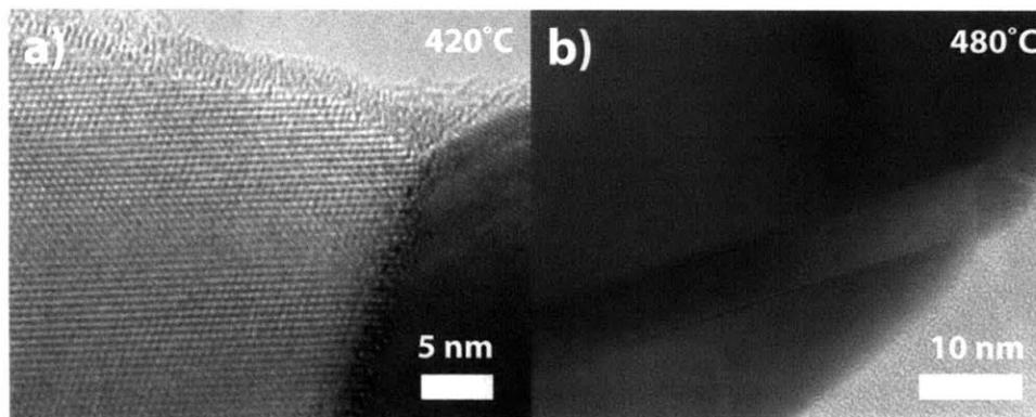
Figure 3-9: High resolution TEM image of a GaAs nanowire grown at 420°C. b) Bright-field TEM image of twinning in a nanowire grown at 480°C.
