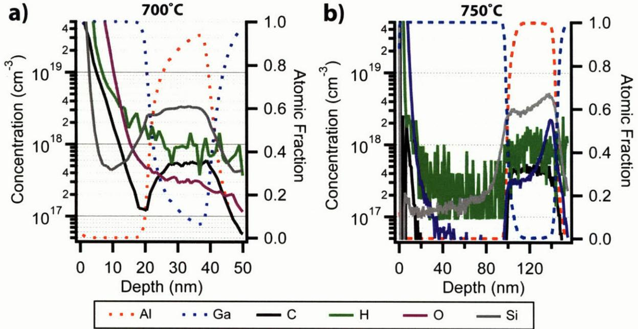
Figure 5-3: Secondary Ion Mass Spectroscopy data for n-GaAs/n-AlGaAs thin-film growth a) 700°C and b) 750°C
