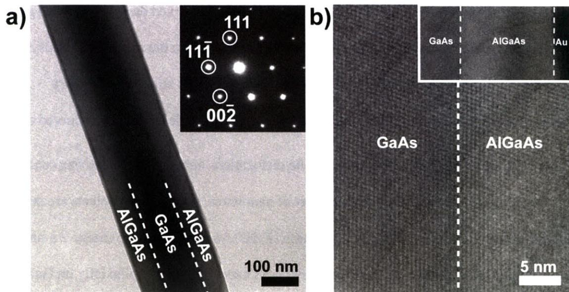
Figure 4-12: a) Bright field TEM micrograph of a core-shell nanowire. Inset is selected area diffraction pattern along  $\langle 110 \rangle$  direction. b) Lattice-resolved TEM micrograph of GaAs/AlGaAs interface between the GaAs nanowire and the Au seed nanoparticle. Inset is same image at lower magnification showing relative positions of GaAs, AlGaAs, and Au.
