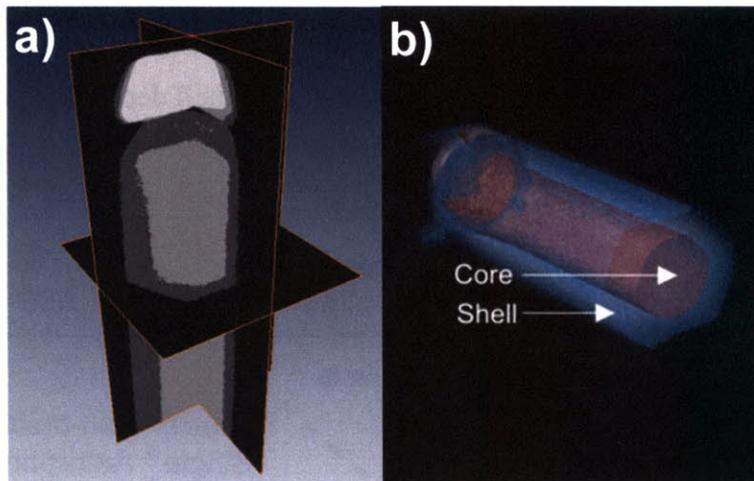
Figure 4-10: a) HAADF STEM images of core-shell nanowires taken at different angles. b) 3D reconstruction of a core-shell nanowire imaged using HAADF STEM tomography. Images courtesy of Dr. Peter Cherns, CEA Grenoble.
