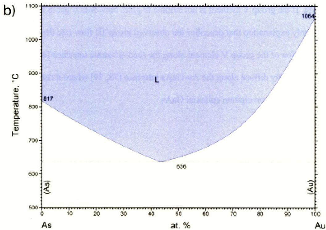
Figure 3-14: Phase diagram for the a) Au-Ga system and b) Au-As system.
