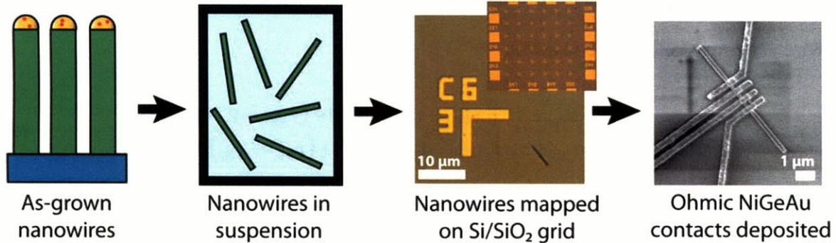
Figure 2-8: Schematic of contacting process showing sonication of nanowires into suspension, deposition of nanowires on the grid, and deposition of contacts.
