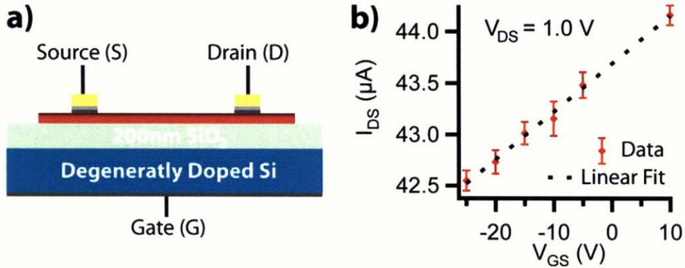
Figure 5-12: a) TLM determination of nanowire and contact resistance and b) back gated IV of the nanowire shown in Figure 5-11 between A-B showing n-type conduction. Error bars are difference between forward and reverse sweep of source-drain voltage.
