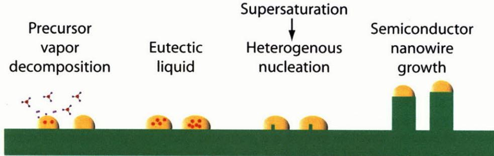
Figure 3-1: Schematic showing the steps of GaAs nanowires by the Au assisted vapor-liquid solid mechanism.
