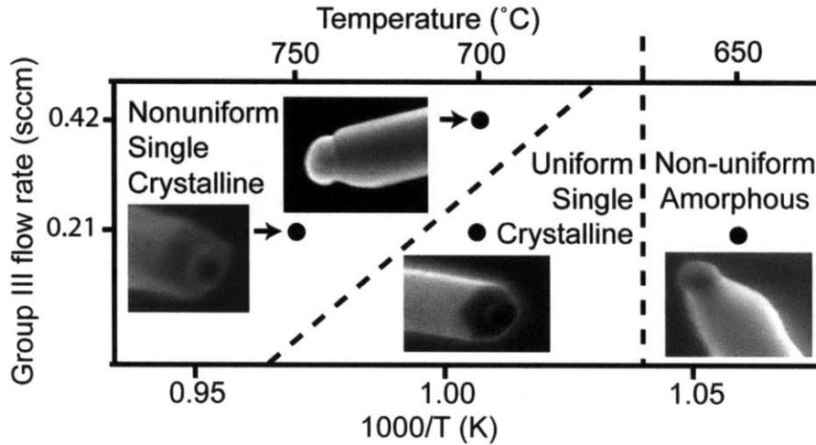
Figure 4-11: Basic zone diagram for shell deposition.
