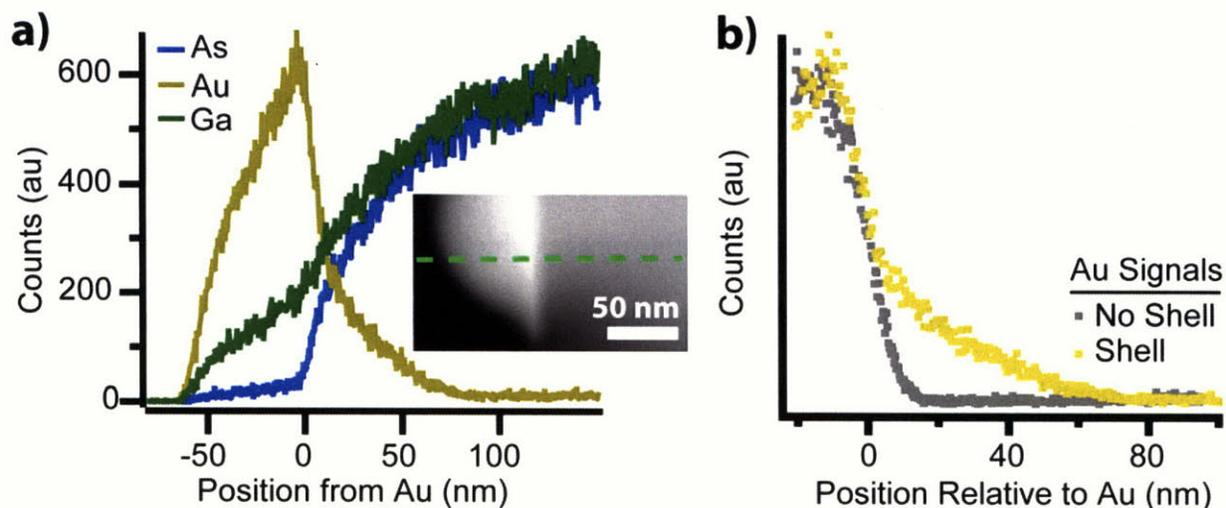
Figure 5-8: a) EDX profiles of Ga, As, & Au at the Au-GaAs interface. Inset is STEM image with linescan shown as the green dashed line b) Comparison of Au EDX signal in a doped shell versus undoped nanowire. The signals were normalized to their maximum Au count.
