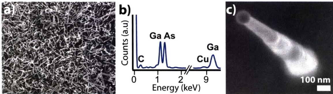
Figure 3-3: a) SEM image of dense forest of VLS-grown nanowires. b) EDX spectrum proving GaAs composition. c) SEM image of a lone nanowire showing tapered morphology.
