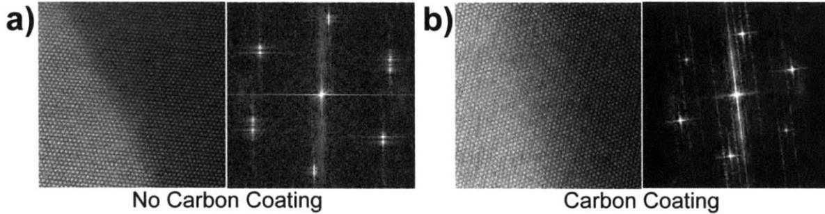
Figure 2-7: HAADF STEM images and corresponding Fourier transforms taken on the same sample a) with and b) without carbon coating.
