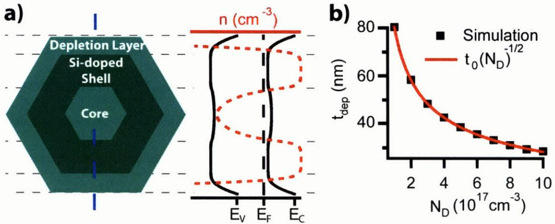
Figure 5-13: a) Schematic of effect of Fermi level pinning on free electron density, and b) thickness of surface depletion layer at different donor concentrations
