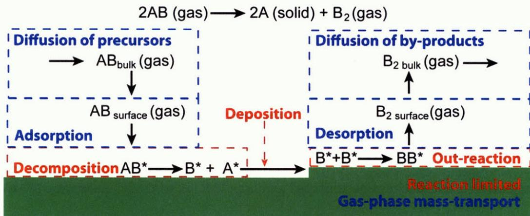
Figure 2-3: Schematic showing the various kinetic steps in MOCVD growth. Steps in blue are categorized as gas-phase mass transport limited steps and steps in red are categorized as kinetically-limited steps. Adapted from [49]
