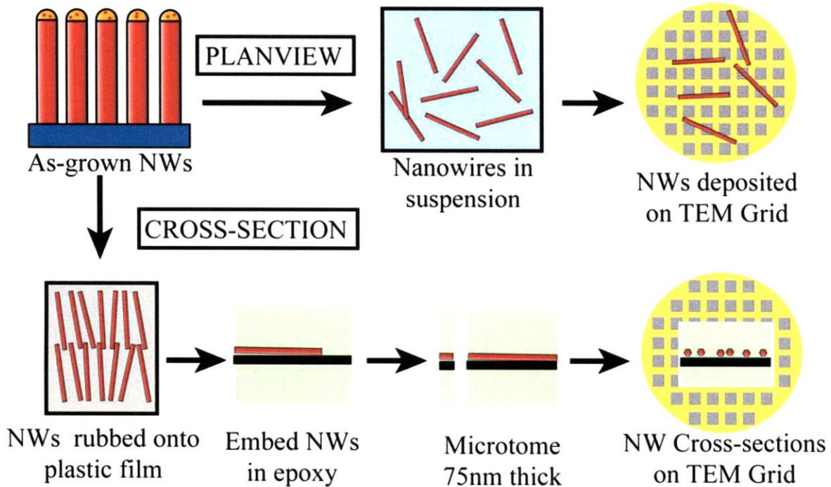
Figure 2-6: Schematic showing the preparation process for plan-view and cross-section nanowire TEM samples.
