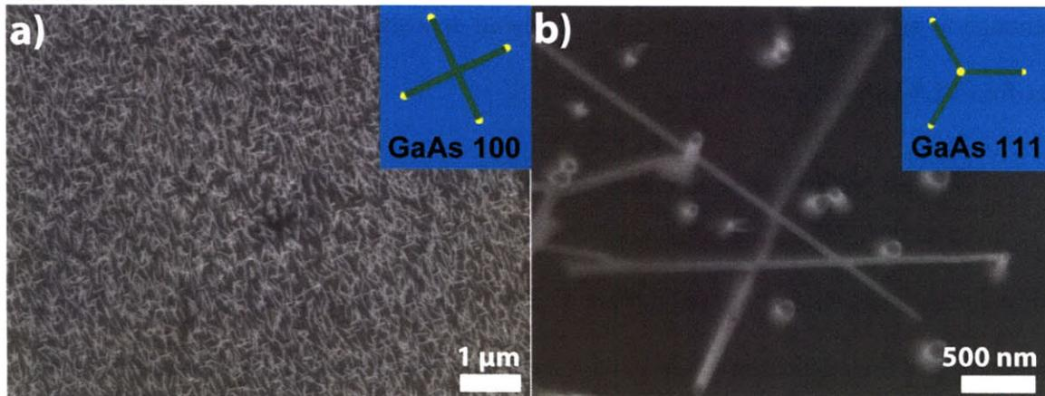
Figure 3-11: Planview SEM images of GaAs nanowires grown on a) GaAs 100 and b) GaAs 111B substrates with observed texturing in inset.
