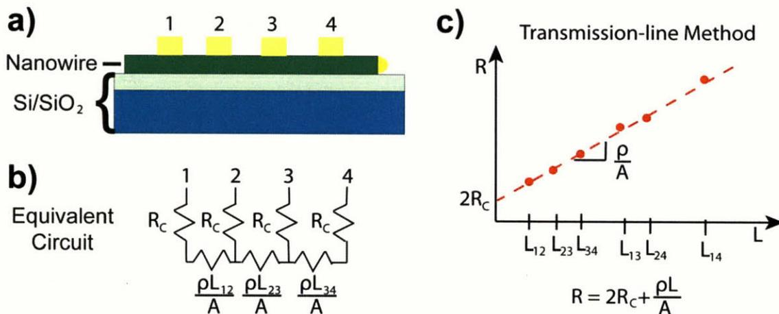
Figure 2-11: Transmission line method measurement on single nanowire. a) Schematic of contacted nanowire. b) Equivalent linear circuit. c) Plot of resistance versus length.
