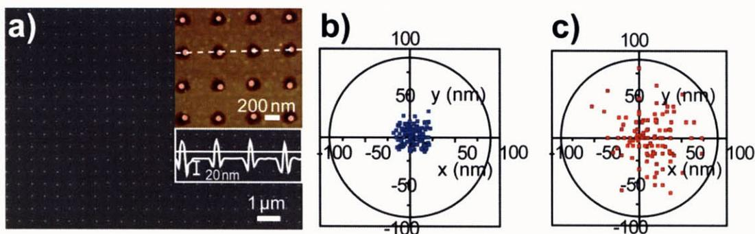
Figure 3-6: a) SEM image of nanoparticles arrays prepared using electron-beam lithography and galvanic reaction after annealing at 600°C for 10 min. Inset is AFM image with height profile. The distribution of nanoparticle positions relative to the mask are shown b) before and c) annealing at 600°C for 10 min.
