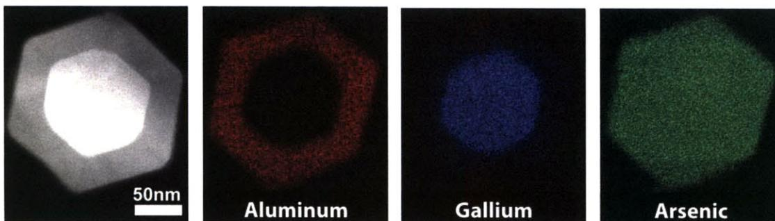
Figure 4-9: High angular annular dark field STEM image of core-shell nanowire cross-section and corresponding chemical maps for aluminum, gallium, and arsenic.
