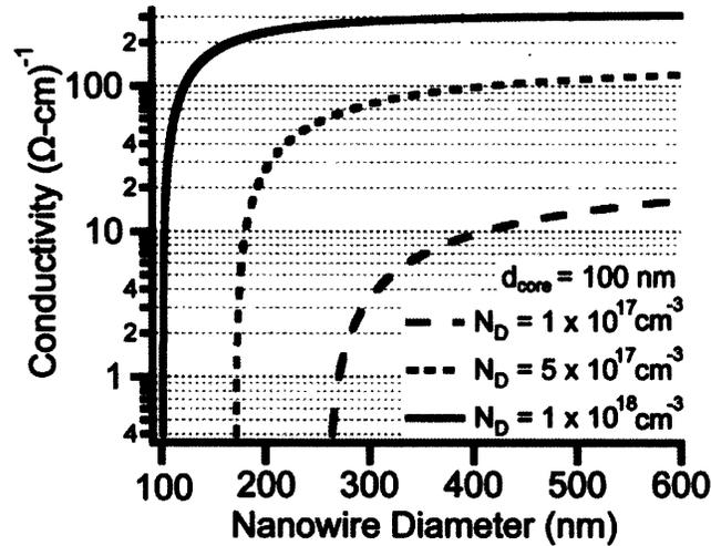
Figure 5-14: Simulated conductivity of core-shell GaAs/n-GaAs nanowires at different shell thickness and carrier concentrations assuming core radius = 50 nm and  $\mu_n = 2000 \text{ cm}^2/\text{V-s}$ .
