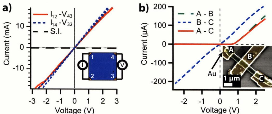
Figure 5-4: Direct current IV data for a) a GaAs (100) control sample and b) a representative GaAs/n-GaAs core-shell nanowire with false-colored SEM of shell contacted nanowire.
