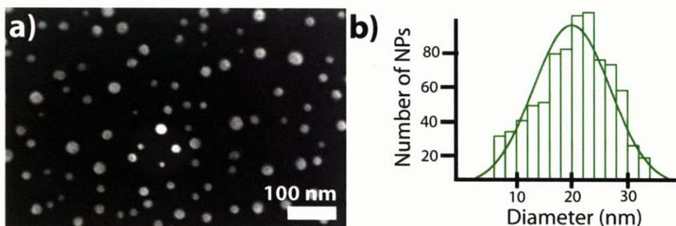
Figure 3-2: a) SEM images of Au nanoparticles resulting from a 6 Å Au film annealed at 600°C. b) Histogram of nanoparticle diameters, after annealing at 600°C, taken from many SEM images.
