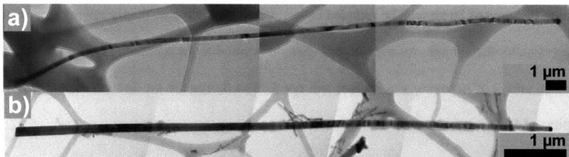
Figure 3-7: TEM images of nanowires grown at 420C (a) and 480C (b).
