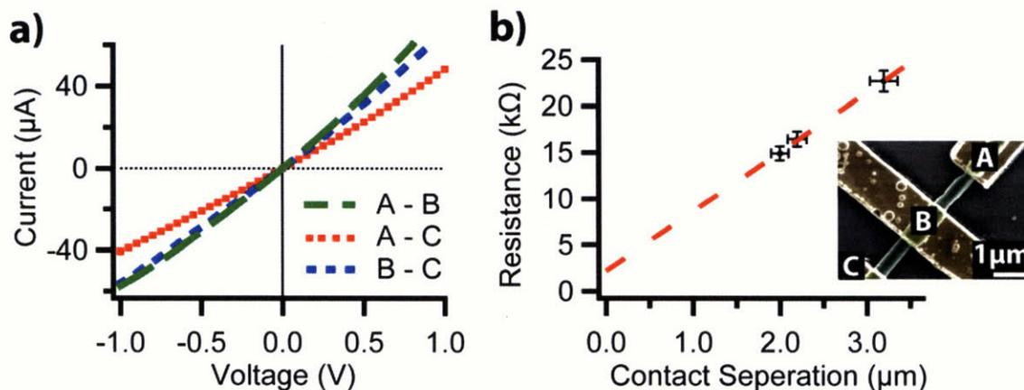
Figure 5-11: a) DC IV measurement of a representative shell-doped nanowire and b) TLM measurement of resistance versus length. Inset is false-colored SEM of contacted nanowire.
