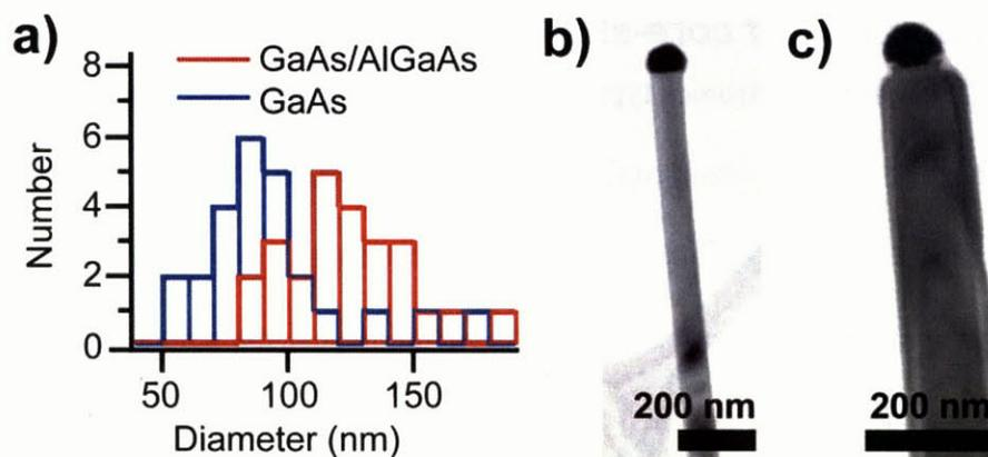
Figure 4-4: a) Histogram of nanowire diameter before and after shell deposition as well as TEM micrographs of nanowires b) before and c) after shell deposition
