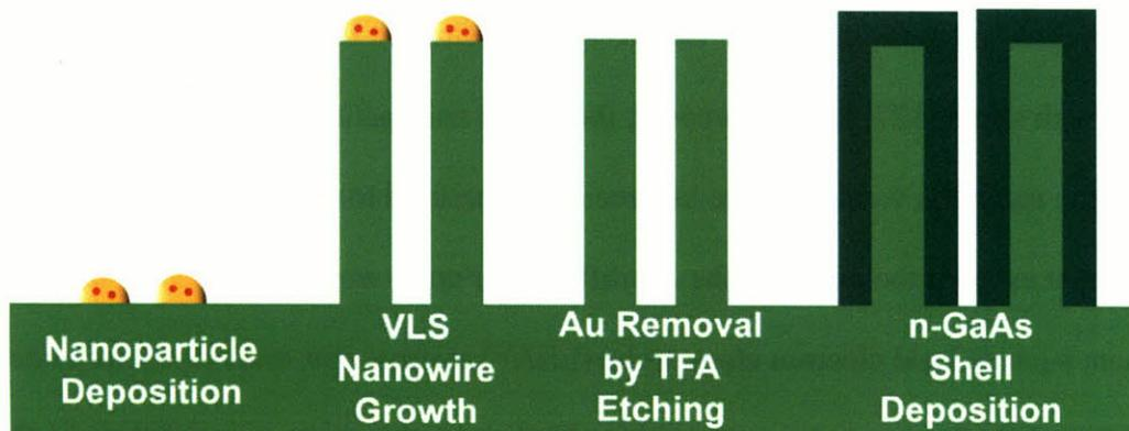
Figure 5-10: Schematic of modified shell doping process including TFA etching process.
