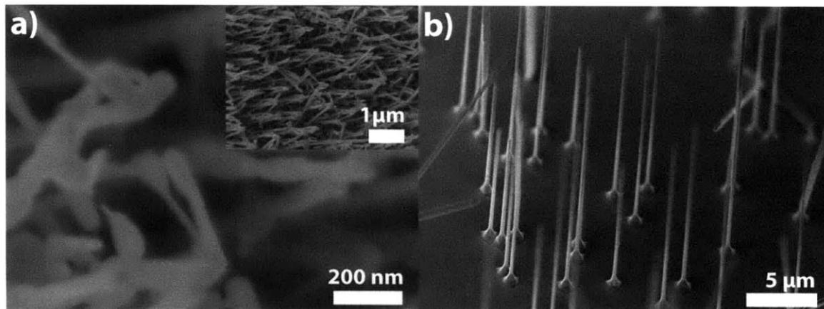
Figure 4-2: SEM micrographs of GaAs/AlGaAs nanowires a) dense nanowire grown at 650°C showing morphological instability, inset is sample at lower magnification and b) sparse nanowire grown at 700°C maintaining morphological stability.
