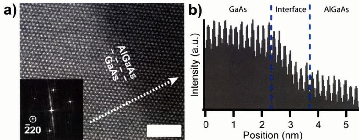
Figure 4-13: a) Lattice-resolve high angular annular dark field STEM image of core-shell interface in cross-section with Fourier transform in inset and b) STEM intensity profile of the core-shell interface along the dashed line in (a). Blue dashed line denotes interfacial region.
