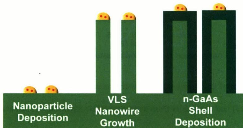
Figure 5-1: Schematic of shell doping process
