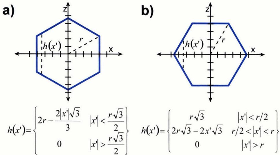
Figure 4-6: Height profile for a hexagonal cross-section nanowire resting on a) a facet corner and b) on a facet.
