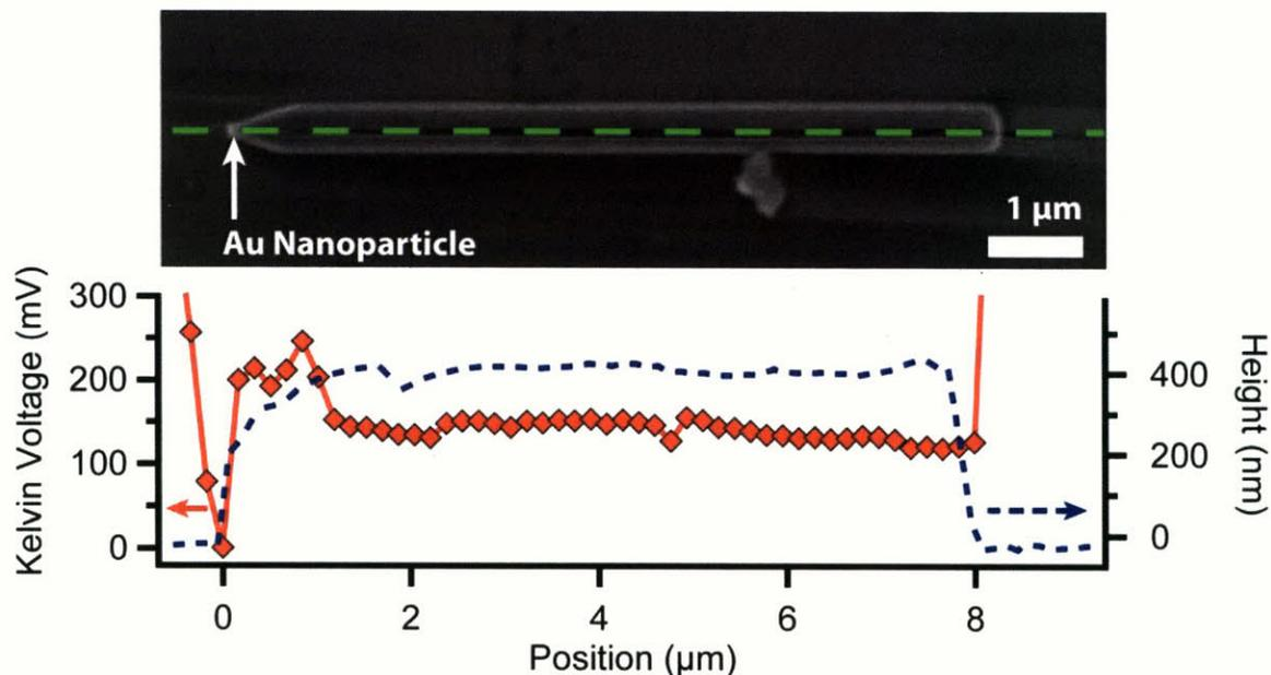
Figure 5-7: Kelvin probe force microscopy of a representative nanowire along the dotted green line pictured in the corresponding SEM image. The red diamonds with connecting line are measured Kelvin potential, normalized to value of the Au nanoparticle and the blue dashed line is the nanowire height profile.
