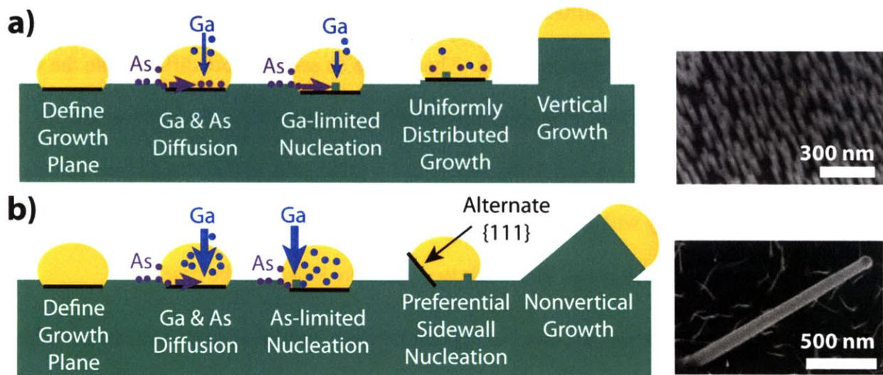
Figure 3-15: a) Schematic of Ga-limited nucleation with corresponding SEM image showing vertical growth. b) Schematic of As-limited nucleation, with corresponding SEM image showing non-vertical growth.
