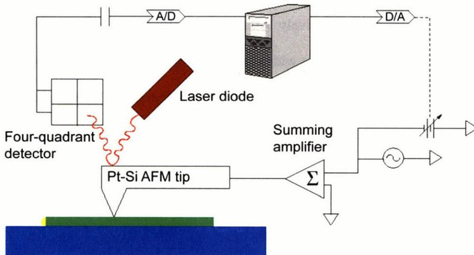
Figure 2-12: Schematic of Kelvin probe force microscopy measurement.
