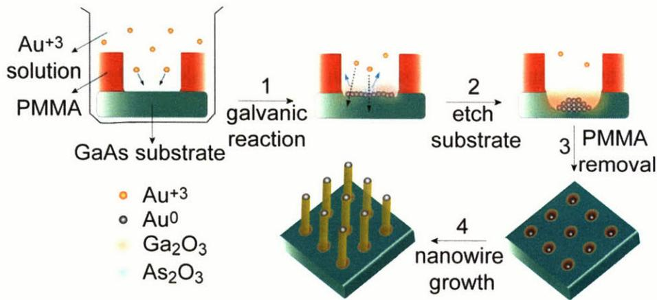
Figure 2-1: The galvanic reaction to deposit Au on GaAs. 1) A patterned substrate is immersed in  $\text{Au}^{+3}$  solution. 2)  $\text{Au}^{+3}$  ions replace  $\text{Ga}^{+3}$  and  $\text{As}^{+3}$  ions producing oxides. 3) PMMA is removed. 4) GaAs nanowires are grown by MOCVD
