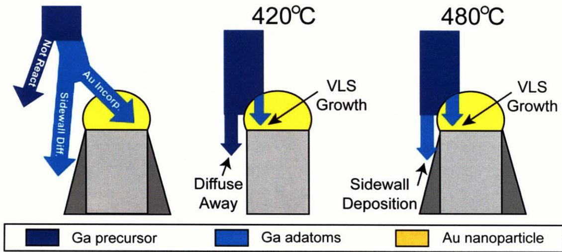
Figure 3-10: Schematic showing the pathways for TMG and how excess Ga adatoms can create radial growth in nanowires.
