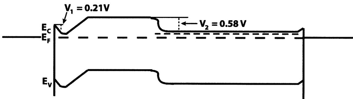
Figure 5-6: Proposed band structure of GaAs/n-GaAs nanowire between contacts A and B.
