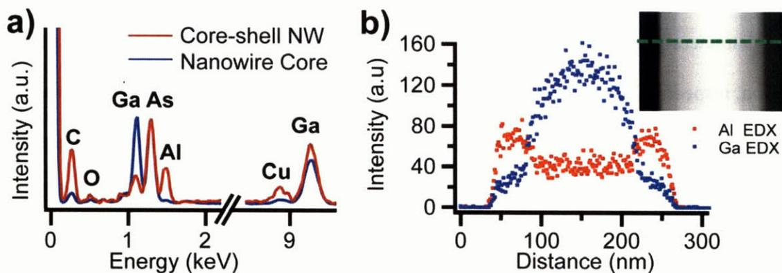
Figure 4-5: a) EDX spectra of a nanowire core and a core-shell nanowire. Signal normalized for As K line. b) Ga and As EDX profiles across the diameter of a core-shell nanowire. Inset is STEM image of core-shell nanowire.
