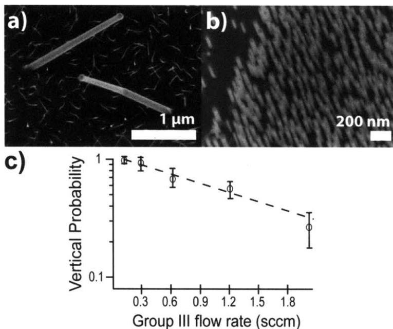
Figure 3-13: Tilted SEM images of GaAs nanowire grown at a) TMGa flow = 2.0 sccm and b) TMGa flow = 0.3 sccm with V/III ratio constant. c) The vertical percentage versus flow rate.
