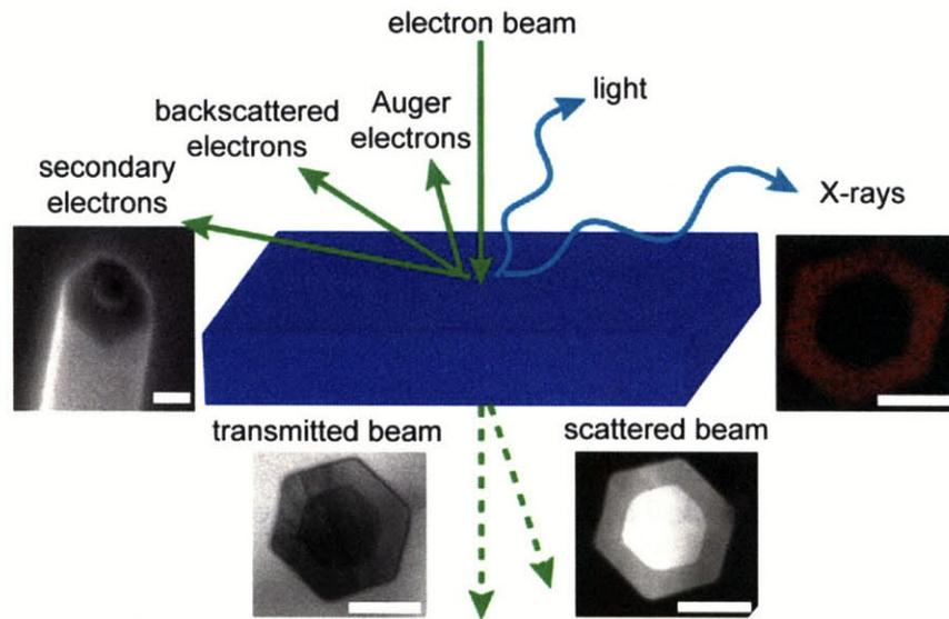
Figure 2-5: Schematic of the various signals that can be produced and collected in an electron microscope. All images have scale bar equal to 100nm. Adapted from [52].
