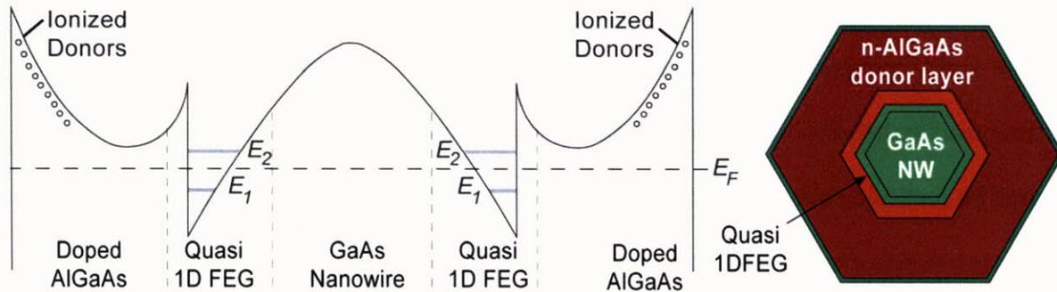
Figure 6-1: Band diagram and proposed structure of core-shell GaAs/AlGaAs structure.
