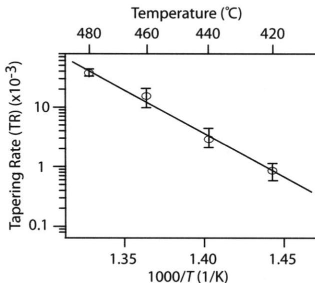
Figure 3-8: The tapering factor plotted on an Arrhenius plot showing shell deposition is a thermally-activated process with activation energy of 56 kcal/mol.
