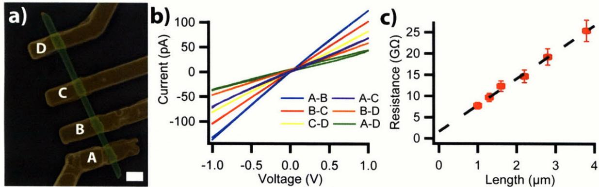
Figure 5-2: Transmission line method measurement of nanowire resistance
