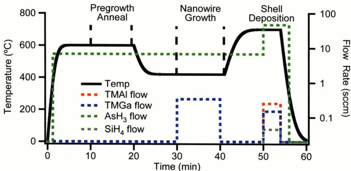
Figure 2-4: Plot of the temperature (left axis) and precursor flow (right axis) profile during a typical core-shell nanowire growth
