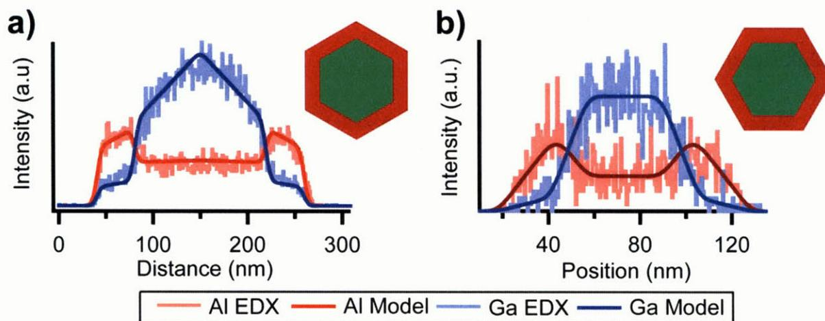
Figure 4-7: EDX profiles for Ga and Al signals in core-shell plotted alongside Gaussian beam broadening model for a core-shell nanowire a) laying on a facet corner and b) laying on a facet sidewall.
