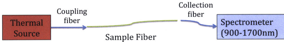
Figure 13: Schematic of transmission bandgap measurements during the fiber draw
