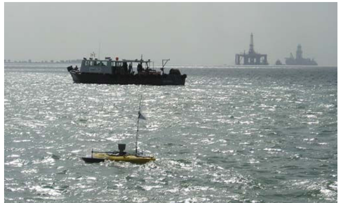
Fig. 1. Autonomous marine vehicles are employed in Singapore Harbor for environmental sensing and modeling, through the Singapore-MIT CENSAM Program. Singapore Harbor presents an extremely challenging environment for such operations, with strong, variable currents and winds, and heavy shipping traffic.
