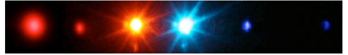
Figure 4. Picture taken with a CCD camera of the images of the second to the sixth harmonic from the near-ir to the uv dispersed by a prism. The ir and uv images are those from the phosphorescent sensors.
