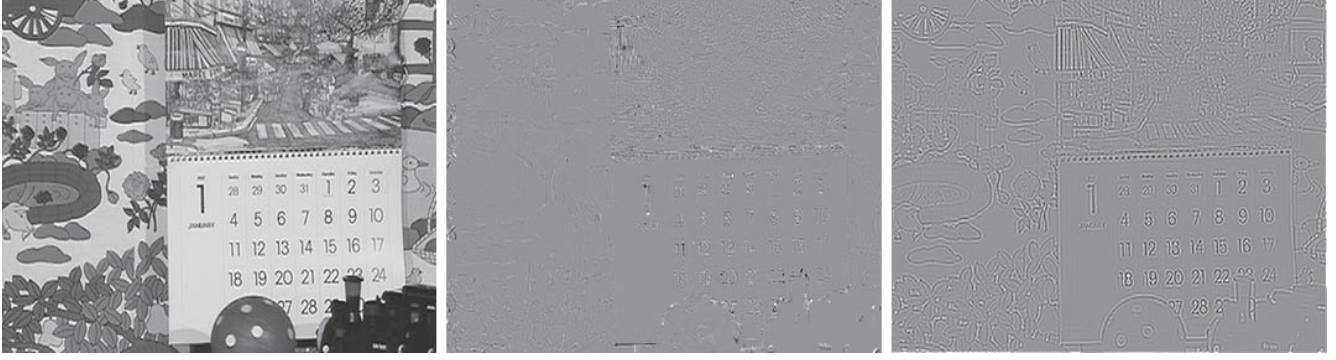
Fig. 1. An image (mobile sequence at CIF resolution, frame 3), its MC-residual (predicted from frame 2) and its RE-residual (predicted from QCIF resolution).
