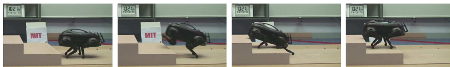
Fig. 2. LittleDog climbs a step dynamically.
