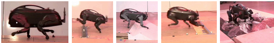
Fig. 5. LittleDog traversing various terrain dynamically.
