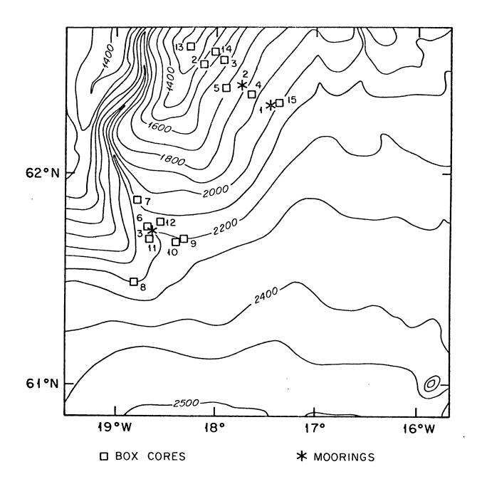
Figure 4.2 Diagram of sediment trap moorings from the northern transect. Traps were located at 503, 103 and 13 mab for Mooring 1 and 493, 103 and 13 mab for Mooring 2.
