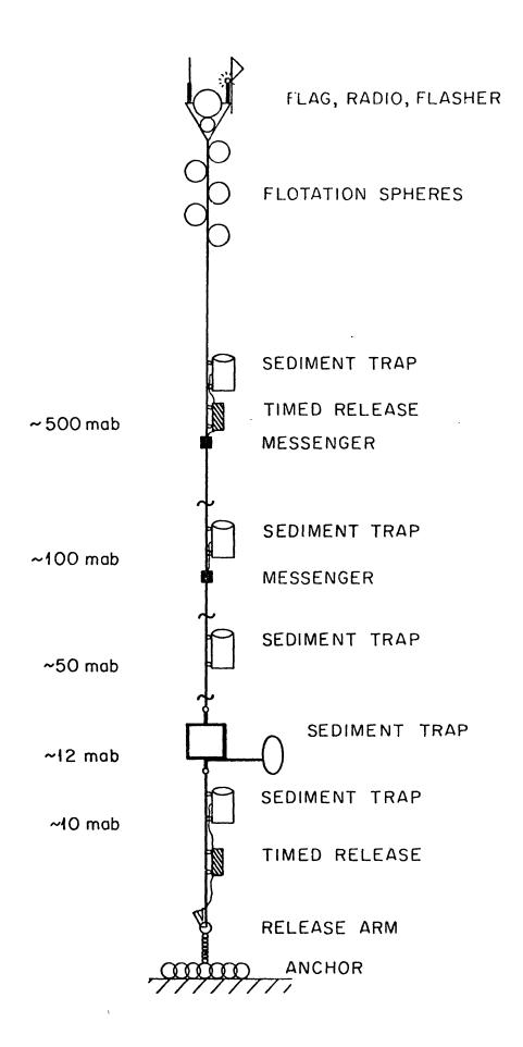
Figure 4.4 The sediment trap used in this study. The trap is a PVC cylinder with a height to width ratio of 2.5. The closing mechanism is a butterfly valve actuated by a timed release.
