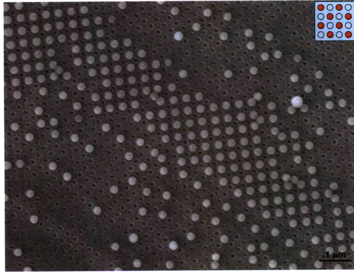
Figure 4-5: SEM image of a template, after convective assembly of 250 nm PS particles from a 0.01-v/v% aqueous suspension. The withdrawal speed of the suspension was 46.1 \mu m/min at 35^\circ C . \kappa^{-1} was 204 nm. This was inferred from conductivity measurement of the solvent. As seen in this image, particles arrange in a sparse pattern. The inset shows a schematic arrangement of particles on the template: red circles denote particles and open circles denote empty holes. Due to the low concentration of the particles in suspension, narrow bands of PS particles assemble on the template.
