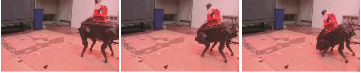
Figure 9: Our quadruped robot scans the surface of a terrain board by bending its legs to sweep the scan line of a back-mounted laser range finder over the terrain surface.
