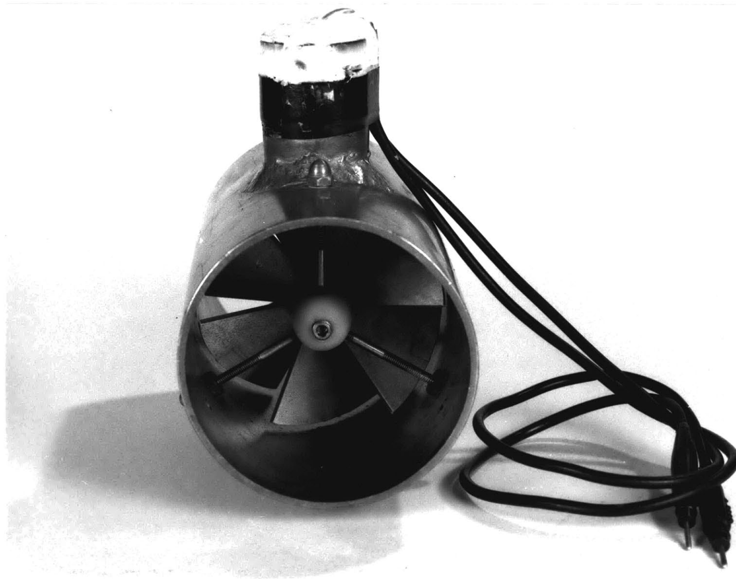
Figure 2. End View of Current Meter
