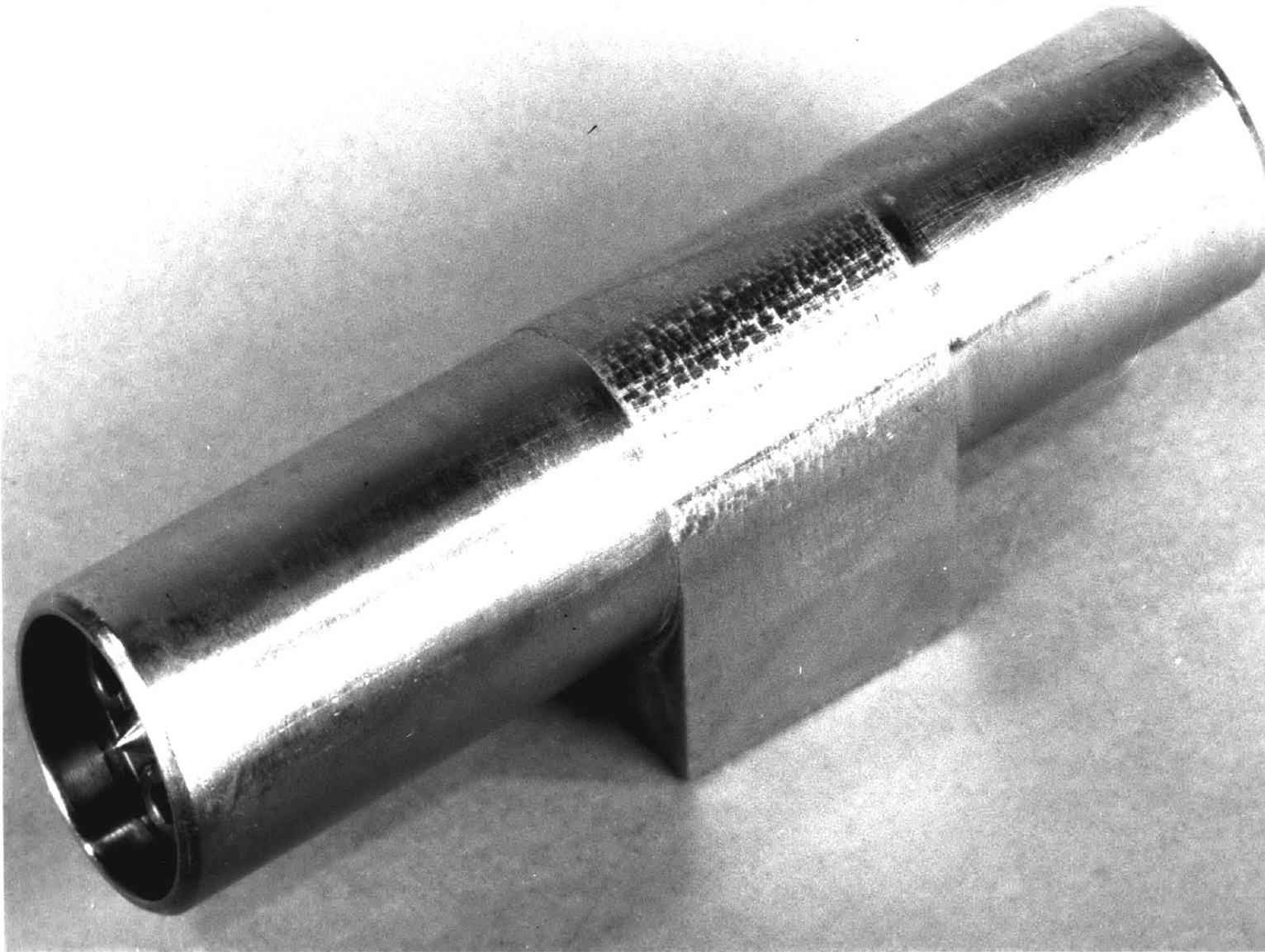
Figure 33. 3/4 View of Modified Cox Instruments Model 12-SCRX Turbine Flow Meter
