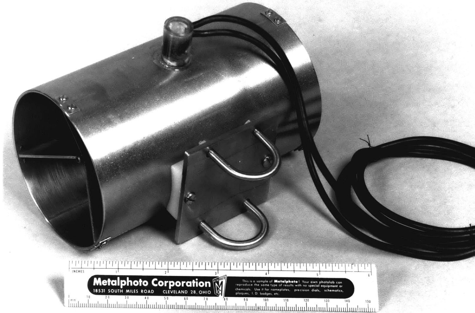
Figure 31. 3/4 View of Braincon Corp. Type 430 Ducted Impeller Current Meter
