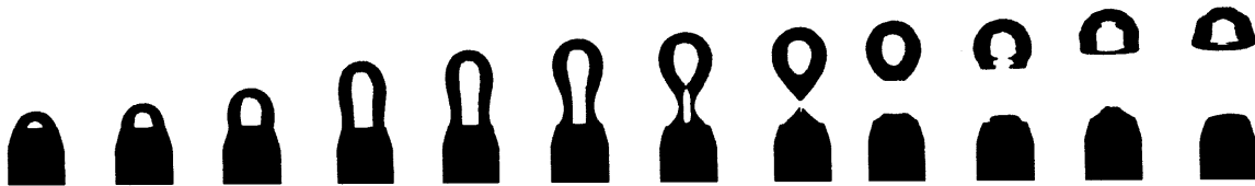
Figure 6: Recorded images of bubble pinch off, nozzle inner diameter 4.00 mm, and film speed 2000 frames/second (Longuet-Higgins 1991).
