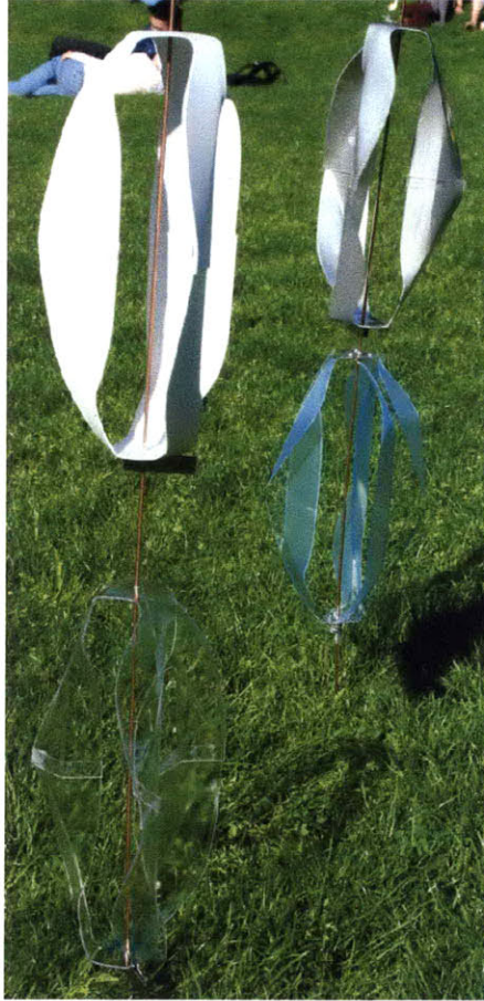
Figure 2: Final product – vacuum-formed vertical axis turbines.
