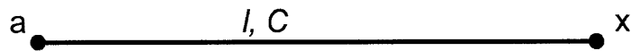
Figure 3.1: A direct-link between node a and node x over a distance l with a channel capacity of C .
