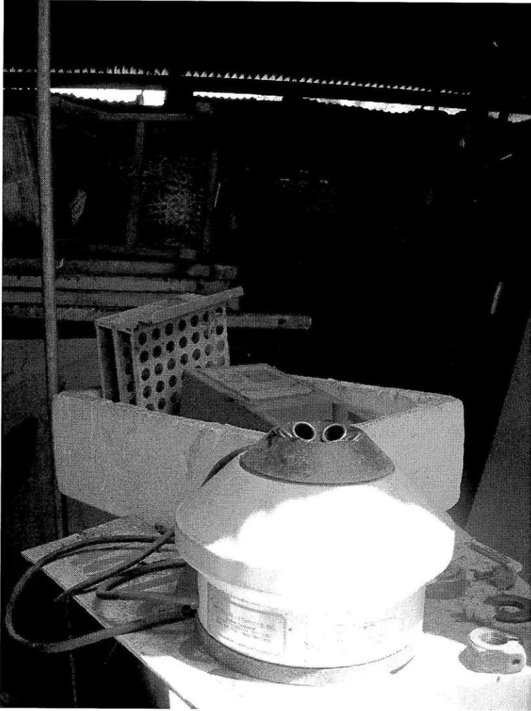
Figure 3. A broken centrifuge that could be re-used if it was connected to a different power source
