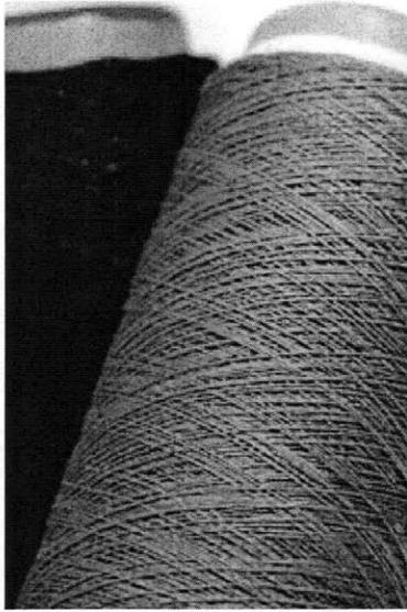
**Figure 4: Silk-wrapped stainless steel core yarn used for knitting and weaving.**
