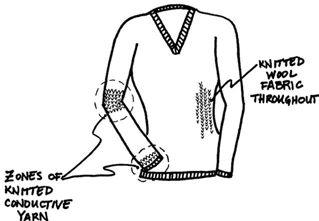
Figure 12: Sketch of a long-sleeve sweater knit with wool and conductive yarns.
