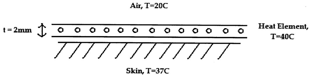
Figure 14: Thermal model of heat element in contact with air and skin.
