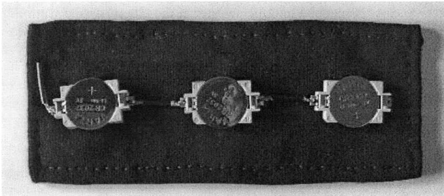
**Figure 18: Wired batteries on wool backing.**
