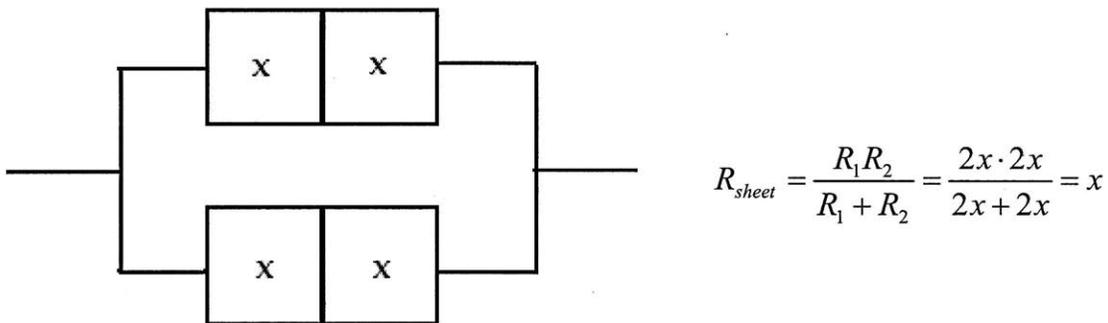
**Figure 7: Sheet resistance as resistors in series and parallel, resulting in units of ohms/square.**
