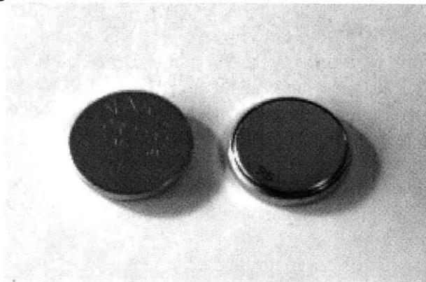
Figure 11: CR 2032 Lithium-Manganese 3V batteries.
