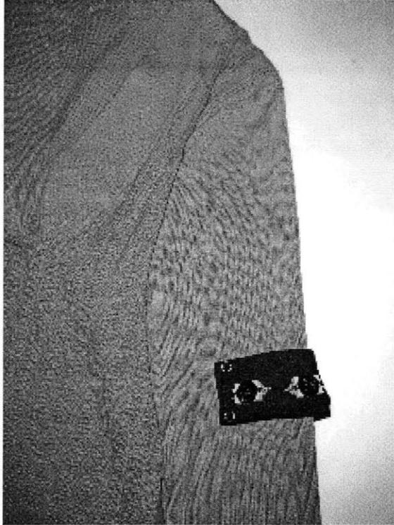
Figure 1: Inside of Therapeutic Heated Sweater with removable battery pack.
