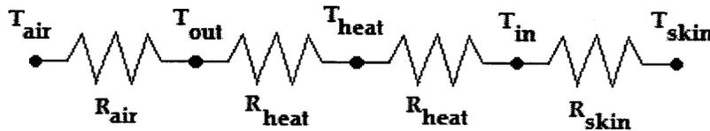
Figure 15: Thermal model as resistors in series.
