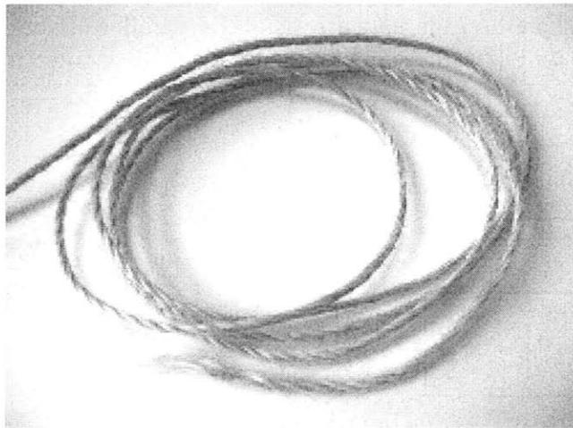
**Figure 5: Schoeller's 10/3 80% Polyurethane, 20% Inox steel yarn.**
