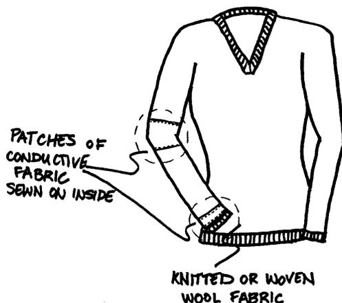
Figure 13: Sketch of a long-sleeve wool sweater with conductive fabric patches sewn on the inside.
