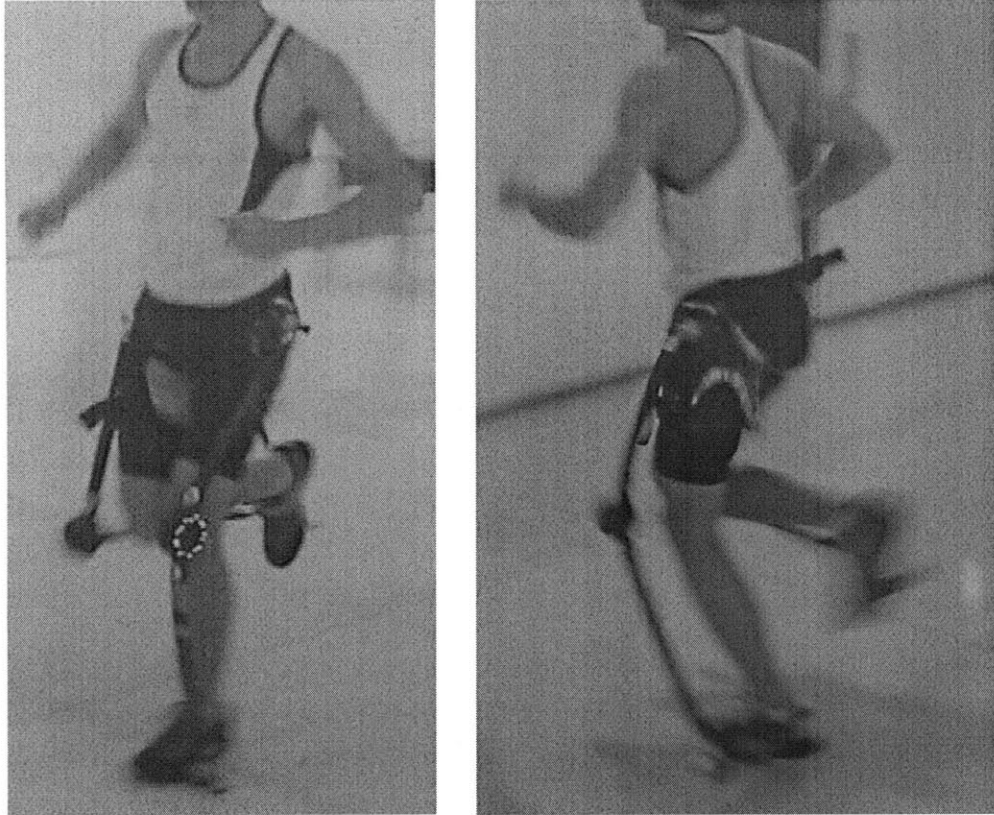
Figure 14: Two views of the exoskeleton during stance phase. Notice how the clutch is locked and energy is stored in the bowing leaf springs.
