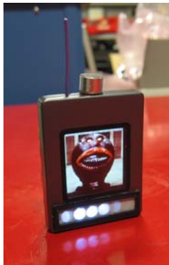
Figure 5. Micro-badge in case with OLED screen
