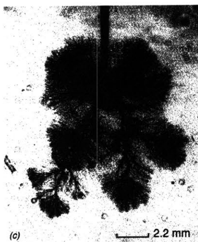
Figure 1.1: Propagation of fast positive streamer in transformer oil in a point-plane electrode geometry under 0.5\mu\text{s} rise time and 85\mu\text{s} fall time impulse voltage. Gap length 27.5mm. Tip radius 30\mu\text{m} ; Crest voltage 178 kV. Schlieren photograph (frame exposure time 8 ns) [1, 2]
