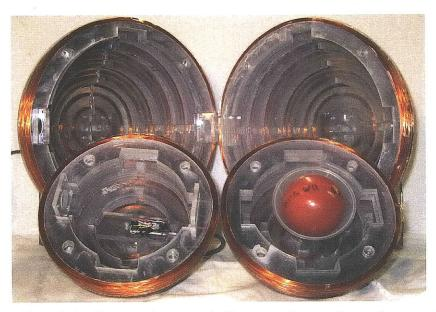
Figure 5-19. Insides of the inner and outer windings are shown. It can be seen that the inner winding has enough space to fit a ferrofluid filled sphere of diameter 10 cm. Image taken from [7].
