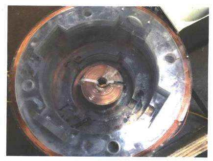
Figure 6-33. Tube inserted in the annulus of third coil (see Figure 6-29) fits inside the inner diameter of the inner fluxball's access tube. This allows for the third coil to be properly aligned along the axis of the fluxball for the numerous experiments conducted.
