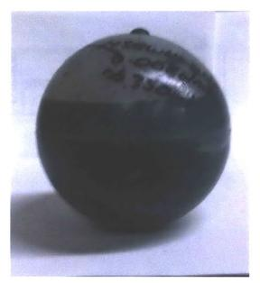
Figure 6-66. Picture of MSGW11 2/3 full sphere of diameter 10 cm. The ferrofluid can be seen to only occupy 2/3 of the volume of the sphere.
