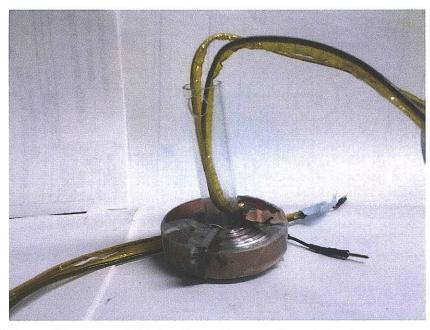
Figure 6-29. Side profile of actual third coil used in experiment. The leads are coated in Kapton insulation tape to prevent conductors from touching if enough current melts the wire insulation. The coil also has a tube fitted to its inner annulus to fit inside the inner fluxball's access hole.
