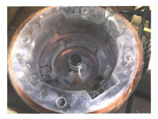
Figure 6-39. Magnet in holder fitted inside upper half of inner fluxball's access hole.
