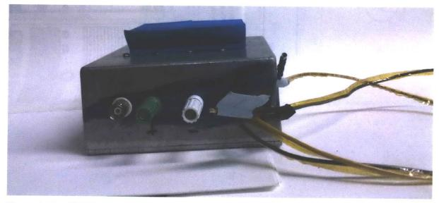
Figure 6-34. 1 $\Omega$  200W resistor in enclosure with heat sinks mounted. BNC connector used to connect the resistor in series with the LVC-5050 amplifier. The leads coated in Kapton tape connect the resistor to the third coil. The banana plug leads allow for the voltage measurement across the 1 $\Omega$  resistor.
