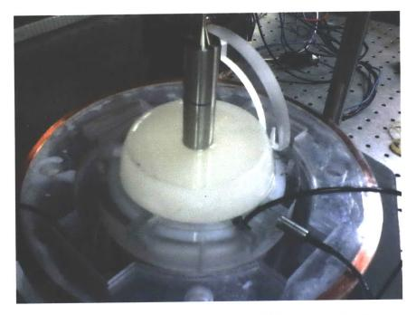
Figure 5-9. Sphere filled with Shell DIALA transformer fluid with disk fitted on LV-1 spindle placed on top of the <sup>3</sup>/<sub>4</sub> sphere.
