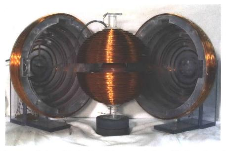
Figure 5-18. An exposed view of the insides of the outer windings. The inner fluxball winding is orthogonal to the outer winding and fits inside the outer winding generating a uniform rotating magnetic field in the region inside the inner fluxball when excited by two phase AC signals. The inner fluxball is slightly separated showing the region inside. Access holes were also made to allow for probes and cables to be inserted inside the inner fluxball. Image taken from [7].
