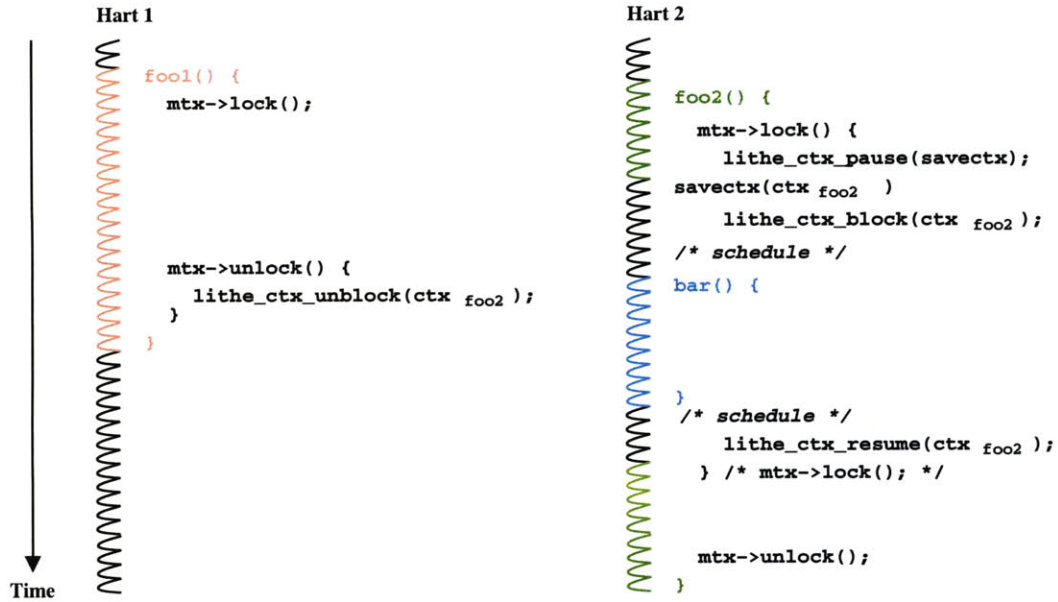
Figure 5-5: An example of how mutual exclusion works with Lithe. foo1 and foo2 are contending for the same mutex. foo1 acquires the mutex first, so foo2 suspends itself and gives the hart back to the scheduler. The scheduler uses the hart to execute bar , then resumes the unblocked context of foo2 .
