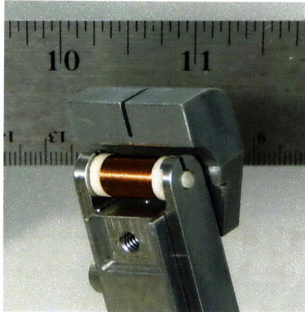
Figure 3-10: A pickup coil is mounted in a limiter with some shielding removed to show the assembly.
