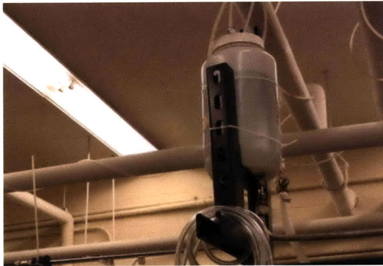
Figure 4.6. ~400 mL accumulator and cool water bath
