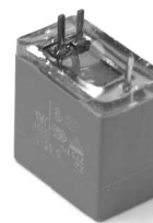
Fig. 21. Photograph of a completed 330 nF integrated filter element with inductance cancellation. The resulting package height is 1.75 mm taller than the original capacitor casing.
