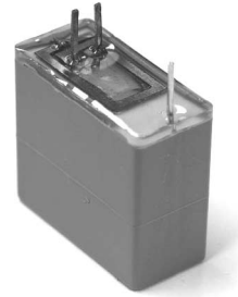
Fig. 25. Photograph of a completed 1.0 \mu\text{F} integrated filter element with inductance cancellation. The resulting package height is 1.2 mm taller than the original capacitor casing.
