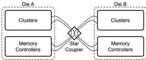
Figure 2: Logical view of a two die system
