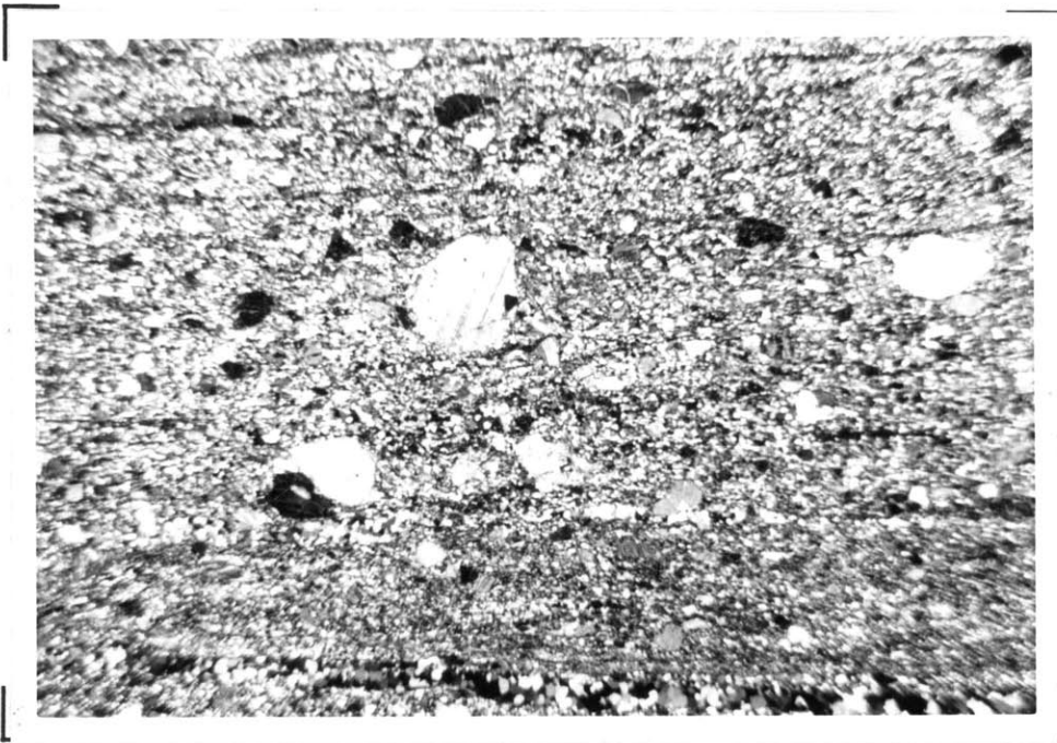
Photograph A8: Granite sample JW-13 ( X polars; field is 13.3 mm wide)
