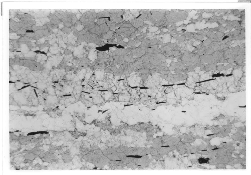
Photograph A28: Granite sample SD-1 ( || polars; field is 13.3 mm wide)
