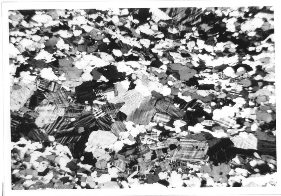
Photograph A14: Granite sample 0-42 ( X polars; field is 13.3 mm wide)
