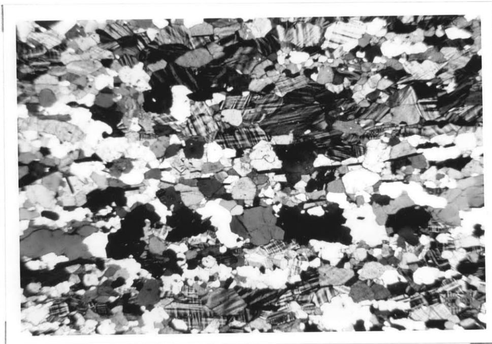
Photograph A29: Granite sample SD-1 ( X polars; field is 13.3 mm wide)
