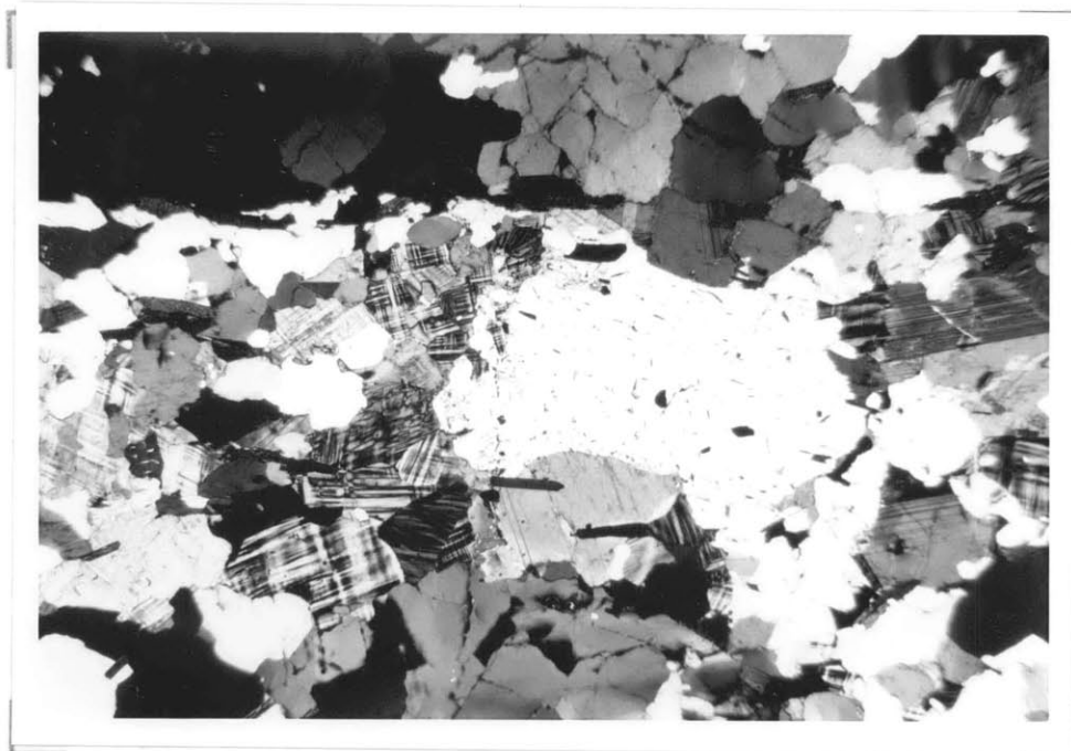
Photograph A20: Granite sample TG-13 ( X polars; field is 13.3 mm wide)
