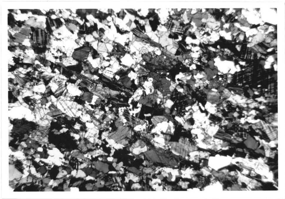
Photograph A22: Granite sample F-4 (X polars; field is 13.3 mm wide)
