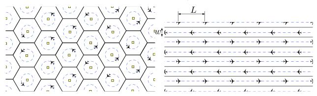
Figure 11. The MC (left) and SL (right) policies with an infinite number of vehicles on an unbounded domain.
