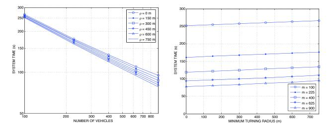
Figure 3. Simulations of the MC policy were run with a square environment of area  $A=9\times 10^{10}~\rm m^2$  and vehicle speed  $v=50~\rm ms^{-1}$ . The performance of the MC policy is plotted as a function of i) the number of vehicles (left), and ii) the minimum turning radius of the vehicles (right). The nonholonomic vehicle densities for the scenarios of all data points shown lie within the range  $0 \le d_\rho \le 0.0056$ .
