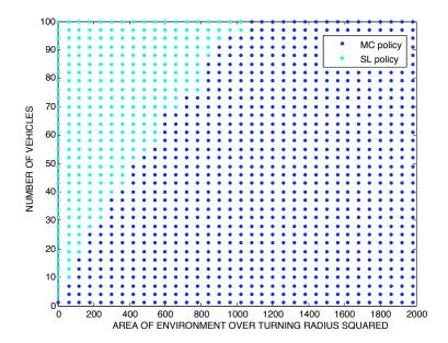
Figure 10. Simulation results aimed at demarcating the phase transition for the case when the environment is a square of area  $A = 4 \times 10^8$  m<sup>2</sup>. The color of the data point signifies which policy had a lower system time for the corresponding values of the parameters.
