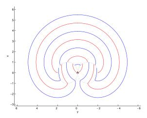
Figure 13. The level sets of the function  $L_{\rho}(g_0, q)$ , for  $\rho = 1$ , shown at increments of  $\pi/4$ . The initial vehicle configuration is represented by the black triangle, and is at coordinates (0,0) heading up. Note that the positive direction of the x axis is up and of the y axis is left.
