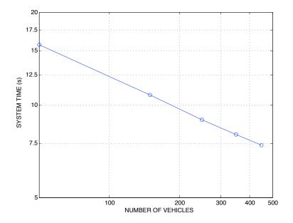
Figure 6. Simulations of the SL policy were run with a square environment of area  $A=9\times 10^6~\text{m}^2$ , vehicle speed  $v=50~\text{ms}^{-1}$ , minimum-turning radius  $\rho=600~\text{m}$ , and m varying from 50 to 450. The nonholonomic vehicle densities for the scenarios of all data points shown lie within the range  $2\leq d_\rho\leq 18$ .
