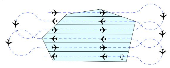
Figure 4. Illustration of the Strip Loitering policy. The segment providing closure of the loitering path (returning the UAVs from the end of the last strip to the beginning of the first strip) is not shown here for clarity of the drawing.
