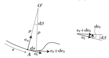
When we move from s to s + ds, the tangent vector changes from  $e_t$  to  $e_t + de_t$ . The change in direction can be related to the angle  $d\beta$ .
