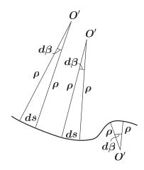
Intuitively, we can see that each infinitesimal arc, ds, can be represented by a circle segment of radius  $\rho$  having its center at the center of curvature. It is clear that both the radius of curvature and the center of curvature are functions of s, and consequently they change from point to point.
