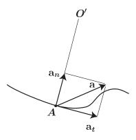
Here,  $a_t = \dot{v}$ , is the tangential component of the acceleration, and  $a_n = v^2/\rho$ , is the normal component of the acceleration. Since  $a_n$  is the component of the acceleration pointing towards the center of curvature, it is sometimes referred to as centripetal acceleration. When  $a_t$  is nonzero, the velocity vector changes magnitude,
