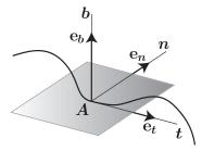
At any point in the trajectory, the position vector, the velocity and acceleration can be referred to these axes. In particular, the velocity and acceleration take very simple forms,
