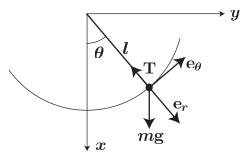
We can formulate the problem in polar coordinates, and noting that r = l (constant), write for the r and  $\theta$  components,
