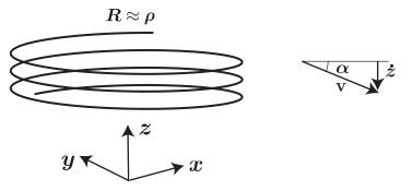
The angle of descent  $\alpha$  is calculated as  $\sin \alpha = -\dot{z}/v$ , or,  $\alpha = -2.72^{\circ}$ . This angle is sometimes called the *pitch* of the helix.
