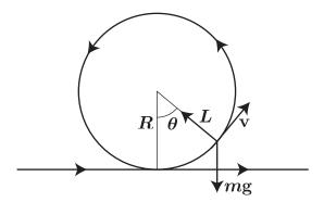
Since the lift,  $\mathbf{L}$ , is perpendicular to the flight path, we have that the force on the aircraft, in normal and tangential components, is
