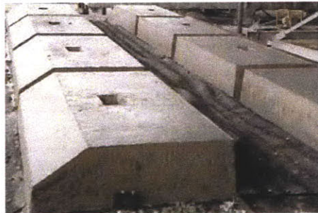
Figure 5.7: Series of mat segments to employ offshore for scour prevention, (Flexmat Gravity Anchor).
