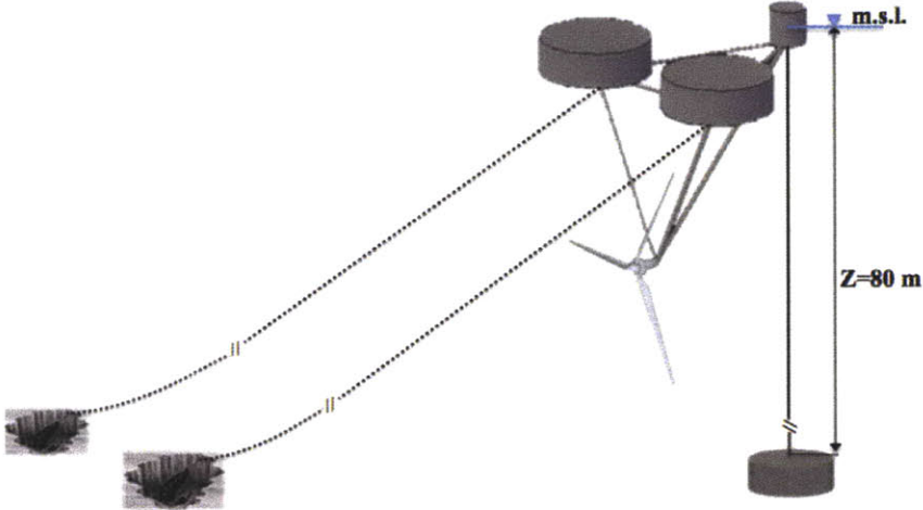
Figure 4.7: Three-platform floating structure bearing a horizontal-axis turbine.
