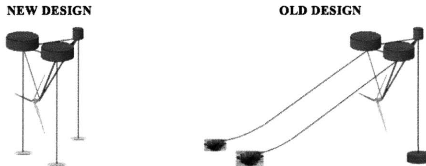
Figure 6.1: New and Old design for the anchor system that keeps the floating structure stationary.
