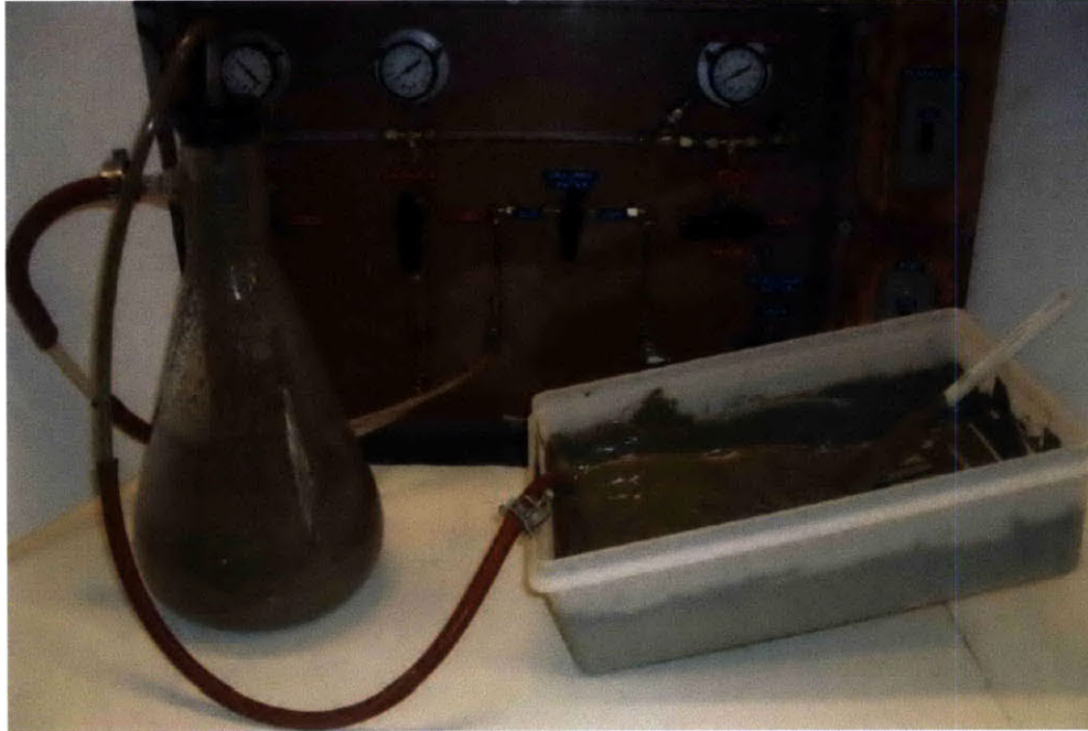
Figure 4-6: Vacuum setup to de air the RBBC slurry (Abdulhadi, 2009)
