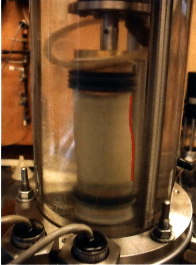
Figure 4-36: Unstable structure causing the specimen to lean to one side during saturation when there is a top cap with no recess for lateral stability
