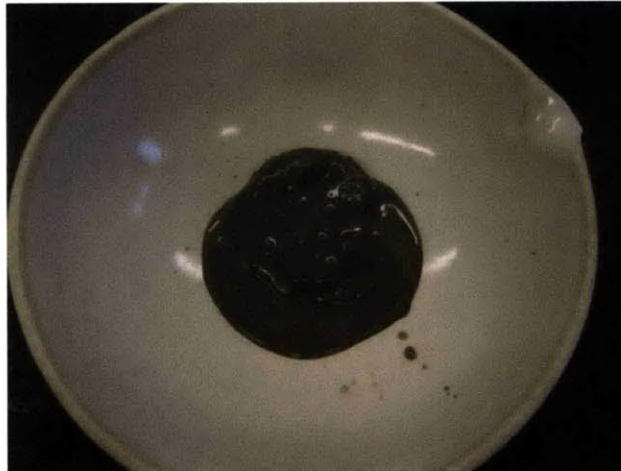
Figure 5-18: Post consolidation behavior; a) CRS specimen extrusion into evaporating dish, b) material behavior after one blow to evaporating dish, c) material behavior after 5 blows to evaporating dish
