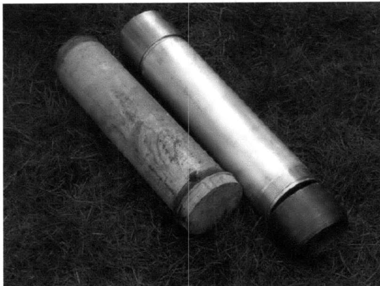
Figure 3-9: “Double” U 100 tubes (Standard Ireland-UK U100 or U4 sampling tubes. Crude cutting shoe shown on right hand side) (Long, 2007).
