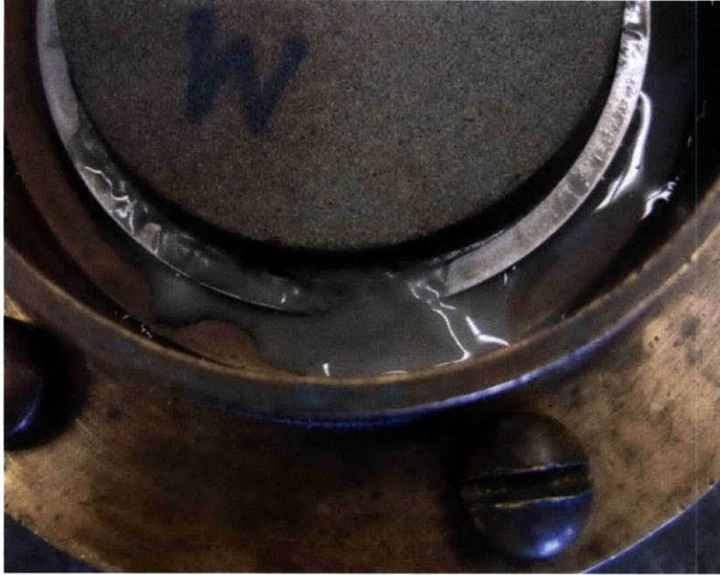
Figure 4-23: “Blow holes” resulting from a high water head
