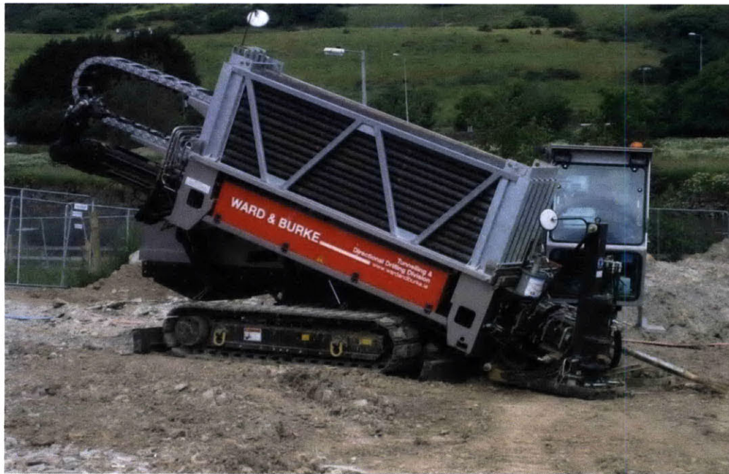
Figure 2-23: Directional Drilling equipment used in Skibbereen
