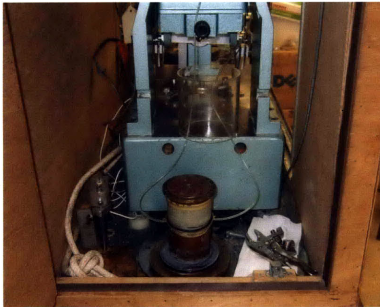
Figure 4-29: Connection of the drainage lines for saturation: (a) schematic, (b) photograph
