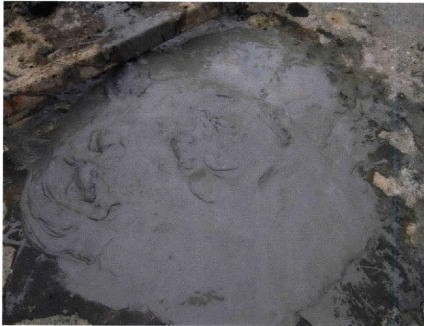
Figure 2-37: Excavated silt from the shell and auger method.
