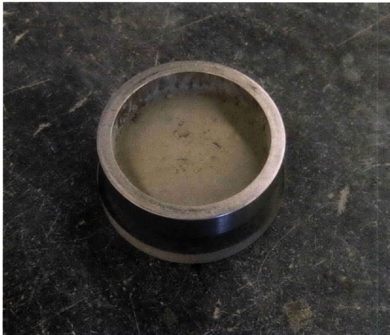
Figure 4-24: Undercompaction in CRS specimen ring from top to bottom using recess tool underneath the specimen ring
