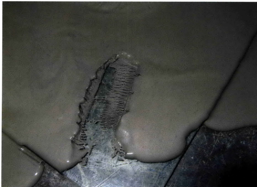
Figure 4-12: Cut through dense material with razor blade after extrusion flow
