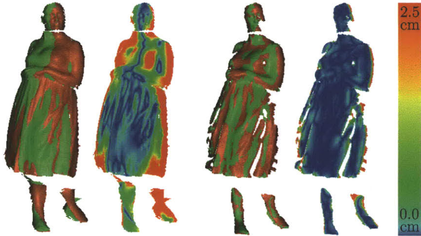
Figure 3-7: The integrated surfaces before matching (left) are far from each other, while the deformed surfaces after matching (right) are much closer to each other. Within each pair, the leftmost visualization shows the two meshes (in different colors) overlaid on each other, while the rightmost visualization is a color-coding of mesh-to-mesh distance.
