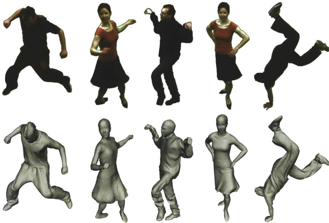
Figure 2-10: Background-subtracted video frames (top) and the corresponding recovered shapes (bottom) for three subjects in five sequences.
