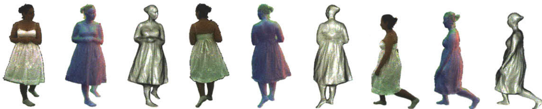
Figure 3-1: Our system rapidly acquires images under varying illumination in order to compute photometric normals from multiple viewpoints. The normals are then used to reconstruct detailed mesh sequences of dynamic shapes such as human performers.
