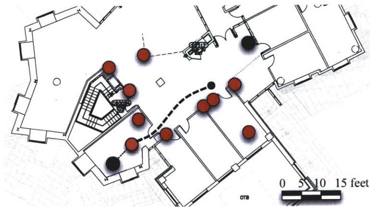
Figure 3-5: Evaluation testbed of software radio nodes: light (red) shaded nodes are senders; black nodes are receivers. The thick dashed line shows the approximate path of the sender in mobility experiments.
