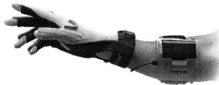
Figure 3-1: Wireless CyberGlove II motion capture data glove by CyberGlove Systems
