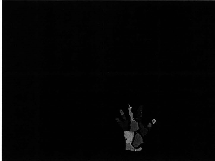
Figure 3-9: Result of color classification after background removal using Method 3 for color transformation
