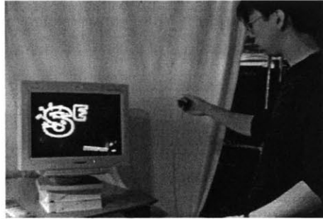
At left, the author performs the letterspace system. As the user moves the two hand sensors, the gestures are mapped to letter changes on the screen.
