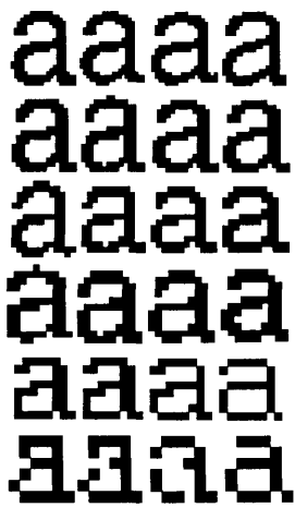
The Helvetica 'a.' From bottom to top, increasing resolution. From left to right, increasingly savvy bitmap rasterizations. (from Hofstadter, p. 597)
