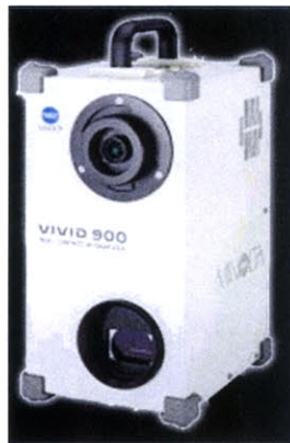
Figure 3.3 The Minolta VIVID 900™ triangulation laser scanner
