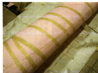
Figure 10 Making the AgoraPhone sculpture out of foam, fiberglass, and epoxy.
