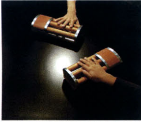
Figure 3-5. InTouch transmits rolling touch by using motors gears and sophisticated control systems.
