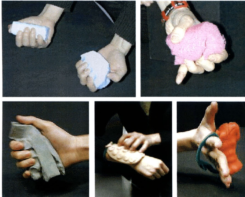
Figure 3-12. Exploration of different form factors using rough prototypes from clay and foam.
