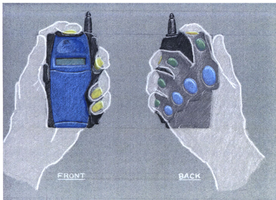
Figure 3-1. Artistic rendering of ComTouch mobile phone holder concept. —Drawing courtesy of James Gouldstone
