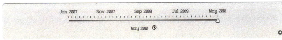
Figure 3-8: This figure displays the history slider that appears in many of the Scratch-Stats visualizations. Using this slider, users can see how the visualization looked during that particular month in history.
