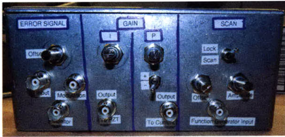
Figure 3-13: Front of the lockbox.
