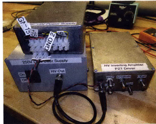
Figure 3-34: The PZT driver setup with a \pm 15\text{V} and 250V power supplies and the PZT driver box.
