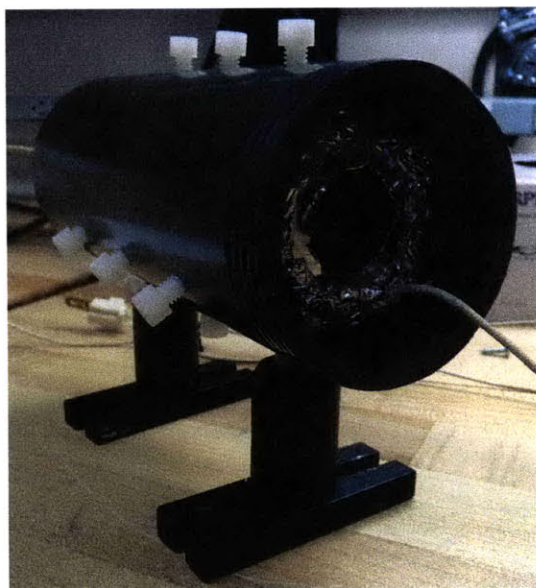
Figure 3-24: The cell is then wrapped in tin foil once more and placed inside the insulating PVC tube which is also attached to Thorlabs mounts.
