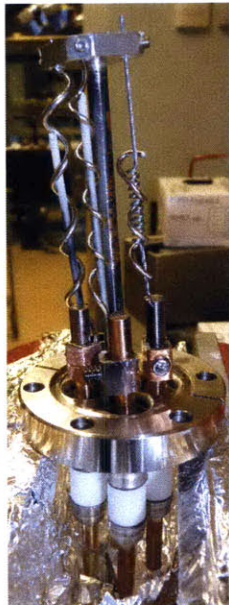
Figure 4-15: Feedthrough with three different attempts to sublimate Zr From left to right: Heating by running current through a 1 mm diameter rod, heating by running current through a 2 mm diameter rod, and heating wrapping a 1 mm diameter rod around a tungsten filament and running current through tungsten.
