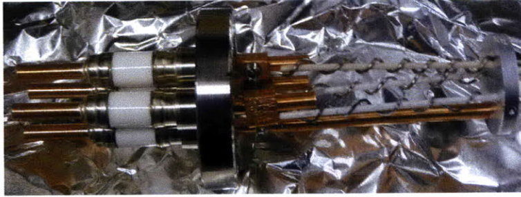
Figure 4-10: The original Ti-Zr-V feedthrough, with the filaments wrapped around ceramic rods and attached to the power line at the base and ground at the top.
