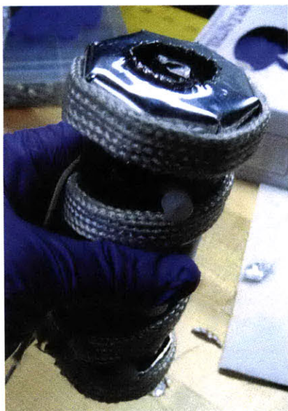
Figure 3-23: The potassium cell, wrapped in tin foil, inside a metal tube, wrapped with a heating band. Windows are glued on two metal caps on the ends.
