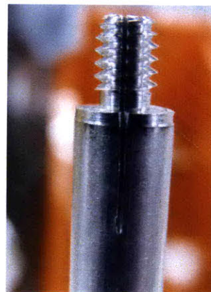
Figure 4-9: The end was turned down to .1640" major diameter for 8-32 threads, .1248" minor diameter thread relief was cut at the top of the threads, and a slit was cut to eliminate virtual leaks.
