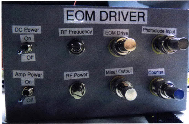
Figure 3-8: Front of the EOM driver box.
