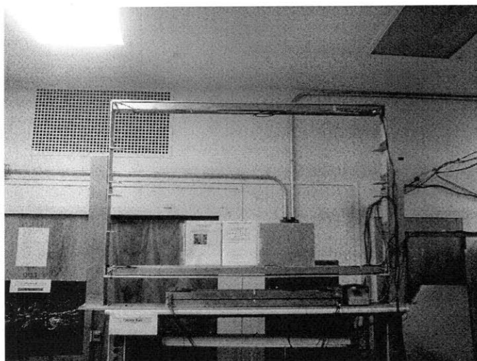
Figure 2-1: The photograph of the apparatus used in this project. Two AMS scintillator counters are mounted in the upper and lower side of the metal frame.
