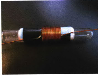
Figure 4-3: Photo of a coil being made.
