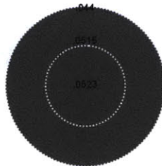
(c) Measured field in the center of the gap (the circle represents the pole piece).
