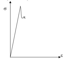
Not expecting the large stress drop, you stop the test abruptly at 'x', and observe that the specimen has **not** fractured and seems to be in fine shape. Although your mind is addled from spending months doing nothing but playing video games, you remember from your 3.14 days that this represents a rapid straining event, and you can think of two possibilities:
