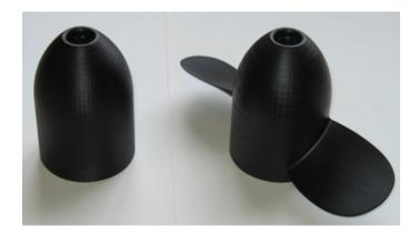
Figure 8-11: Finished hub and propeller.
