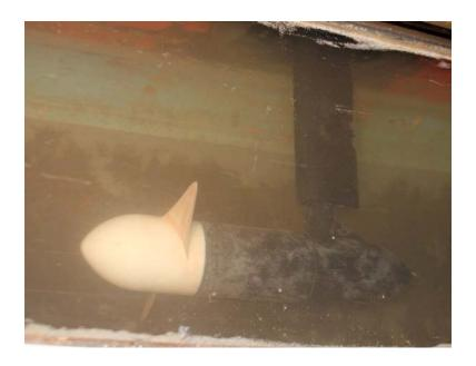
Figure 9-9: Finished turbine in the water tunnel. The flow is still left to right as in the propeller experiments, but the motor housing has been turned around such that the load on the propeller shaft is still compressive.
