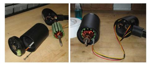
Figure 8-2: Hall-effect sensor installation.
