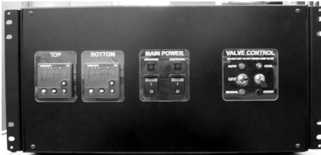
**Figure 4.13** Photo of the temperature control system front panel. The PID heater controllers are at left, and the manual override switches for controlling the coolant flow are at right.
