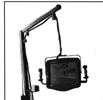
Figure 8.18. The WindowsVR rig has joysticks to register translation. [Absolut, 2002]
