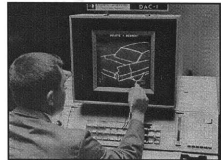
Figure 2.8. In 1959, the DAC-1 (Design Augmented by Computers), developed by General Motors and IBM, became the first interactive 3D computer graphics system.
