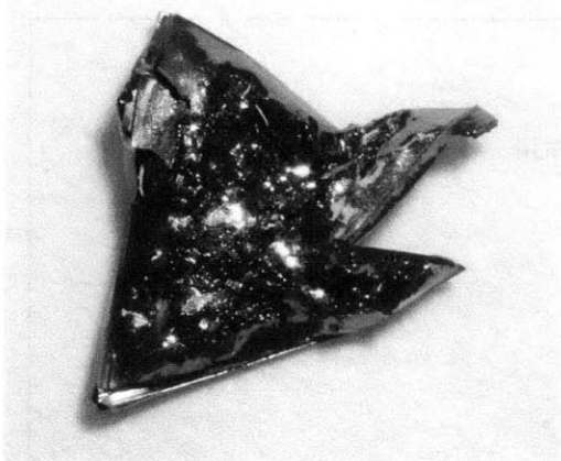
Figure 4-12: Wet oxide-coated sample with “folding” deformation from original shape.
