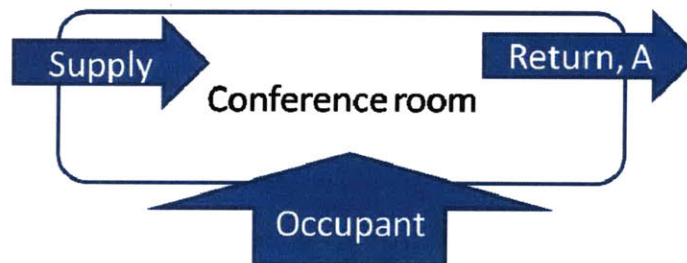
Figure 37 control volume analysis of CO 2 species balance around set of conference rooms
