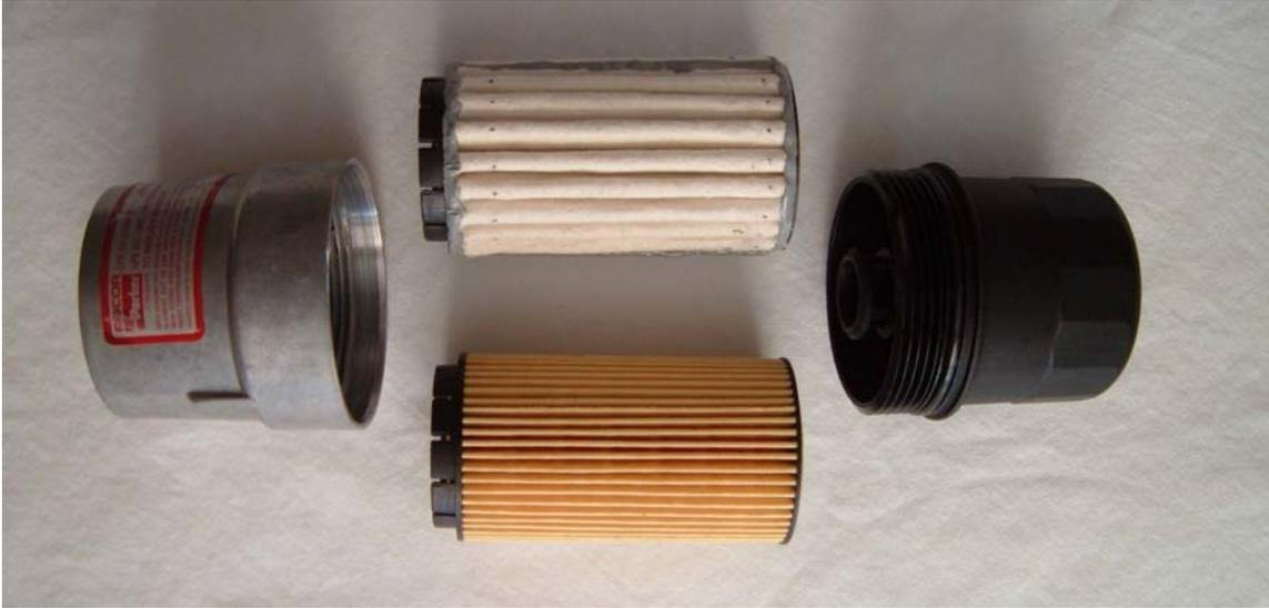
**Figure 5.5** – Both filter elements were mounted in a Racor™ full-flow housing. Both filters contained identical oil volumes and similar flow profiles.
