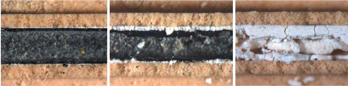
**Figure 2.8** – Typical ash and soot distributions in the channel of a regenerated DPF. The inlet for flow is on the left of the picture. Exhaust passes through to the outlet, on the right of the picture [40].
