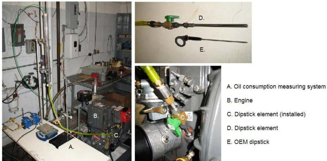
**Figure 3.8** – Pictures of the sump oil sampling system.
