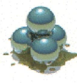
**Figure 3.10** – The contact geometry used during a four ball wear test.
